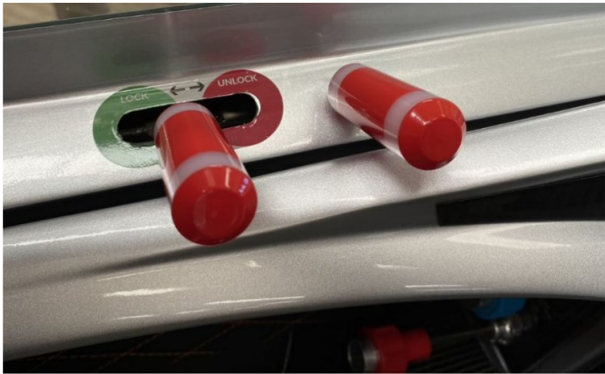
Canopy handle partly locked position when under spring pressure alone
