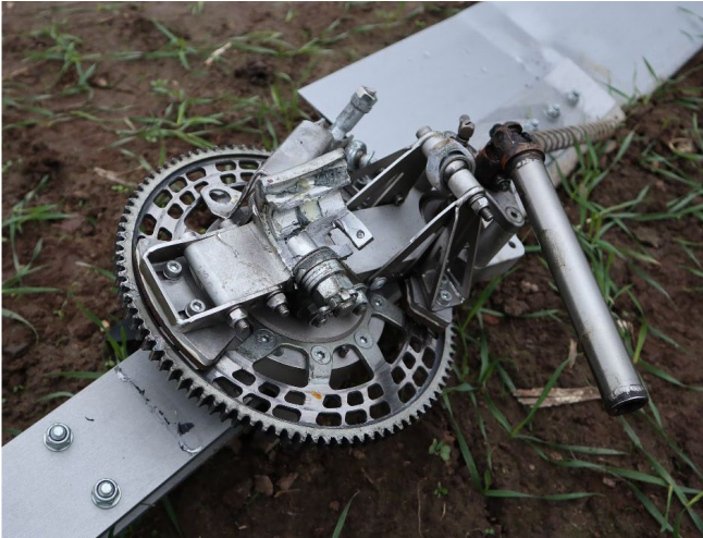
Rotor head showing gimbal block failure, rotor blade deformation and teeter stop contact mark
