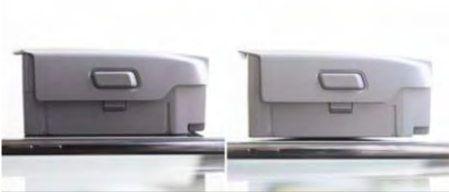
Battery without swelling with a flat underside (left) compared with one with swelling evident (right). (Used with permission)
