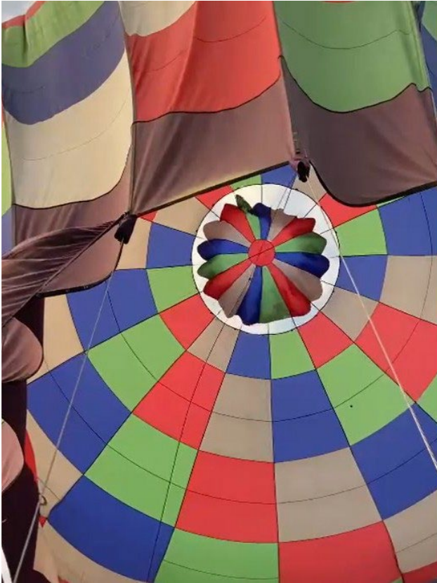
Example parachute in a stalled condition (Looking up through the balloon envelope from the basket)
