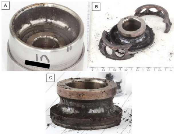
(A) Inboard row, outer race, (B) Inboard row inner race and fractured cage, (C) Inboard row inner race
