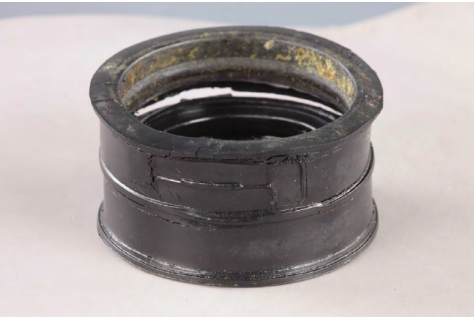
Split carburettor coupling from G-CDFK
