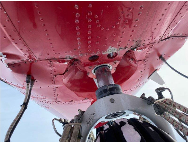
Damage to aircraft skin around the nose gear
