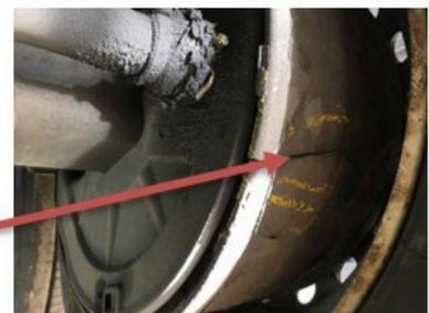
Brake drum fracture = **not acceptable**
