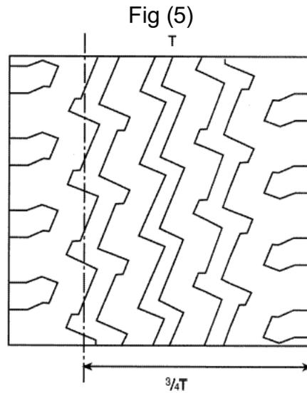
In this case the lateral grooves are the same depth as the circumferential groove and are included in the  $\frac{3}{4}$  measurement.
