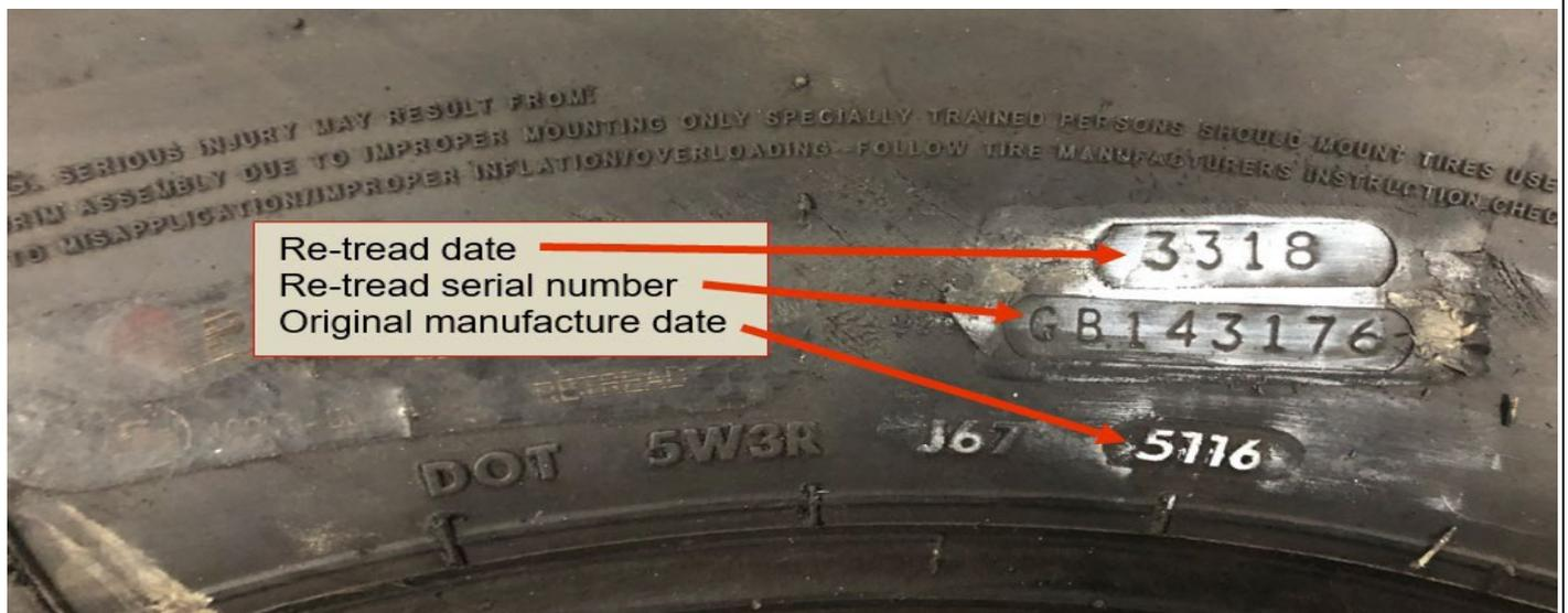
Tyres not displaying a date code would normally be a deficiency. However, date codes are only required to be marked on one side of the tyre so it may not be possible to see the date code on some twin wheel fitments. Under these circumstances you should assume the date code is present and the tyre age is acceptable.
