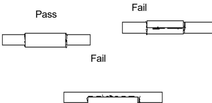
**Guidance on sleeved repairs** of metal brake pipes (sleeving is not acceptable on plastic brake pipes).
