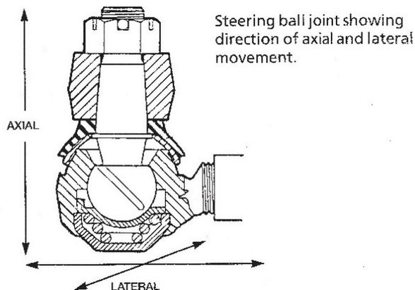
An increasing number of vehicles are now fitted with different types of ball joint, spring loaded or rubber mounted type each having different wear limits (some vehicle may be fitted with both types of joint). The rubber mounted type has a smaller wear limit than the spring loaded type.
