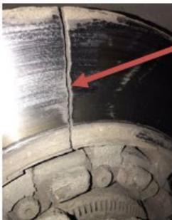
Brake disc fracture = **not acceptable**
