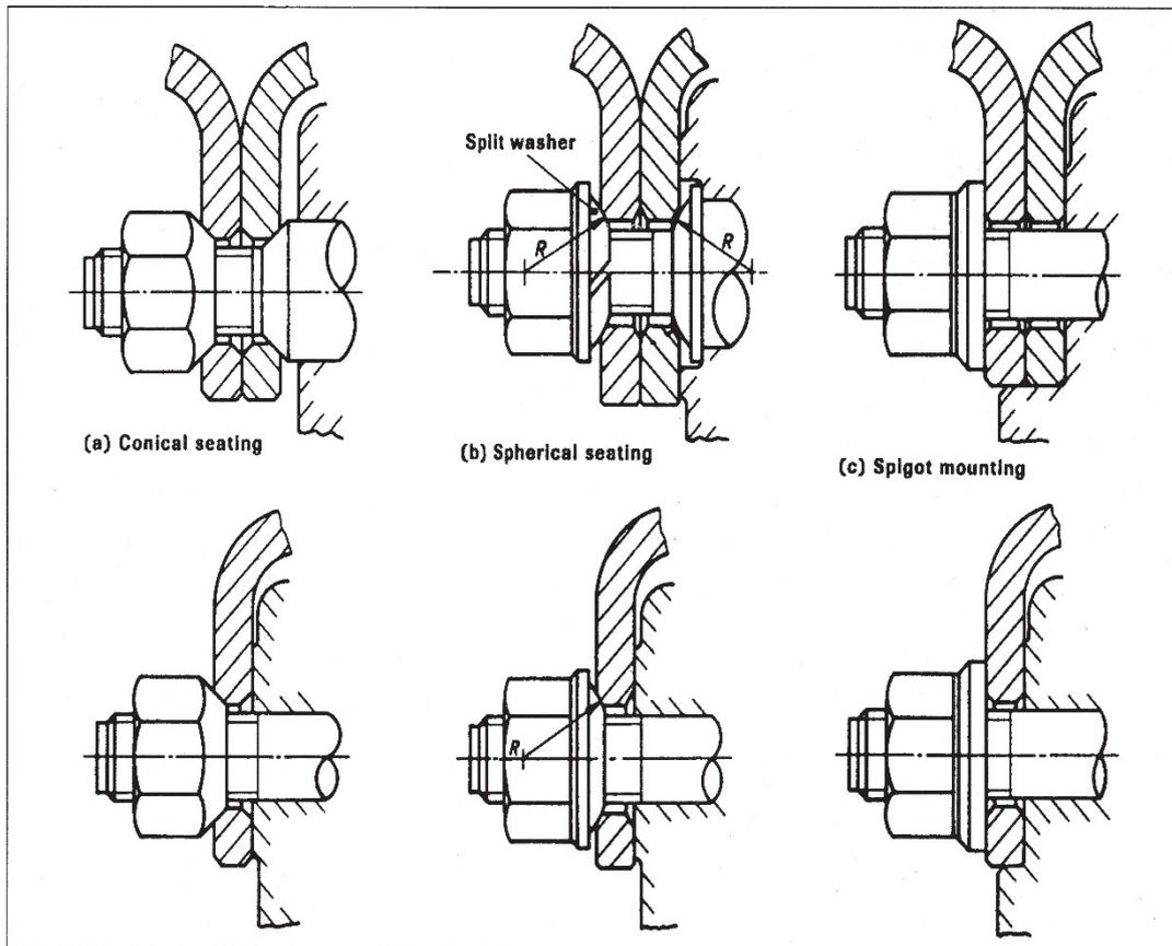
Vehicles with conical wheel fixings **MUST NOT** be fitted with wheels from vehicles designed for use with spherical fixings. (British built vehicles normally have conical wheel fixings).
