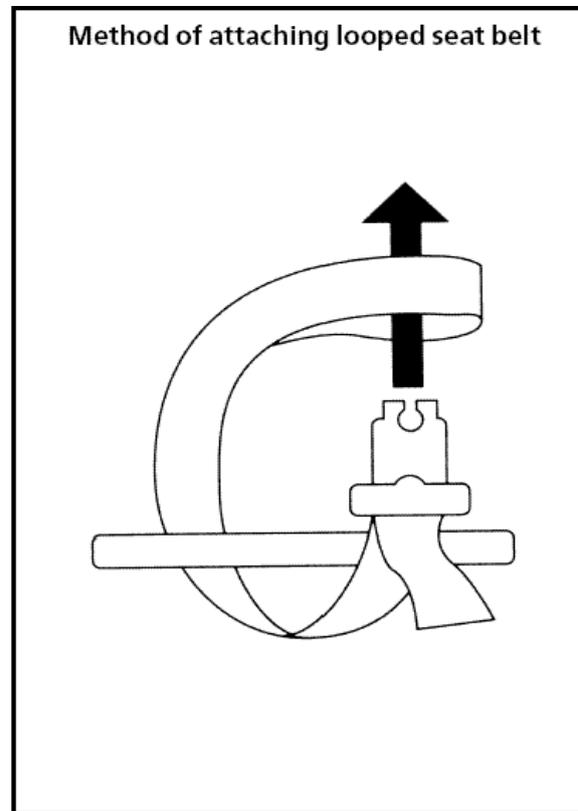
Diagram 2 – Example of a typical clamp bracket
