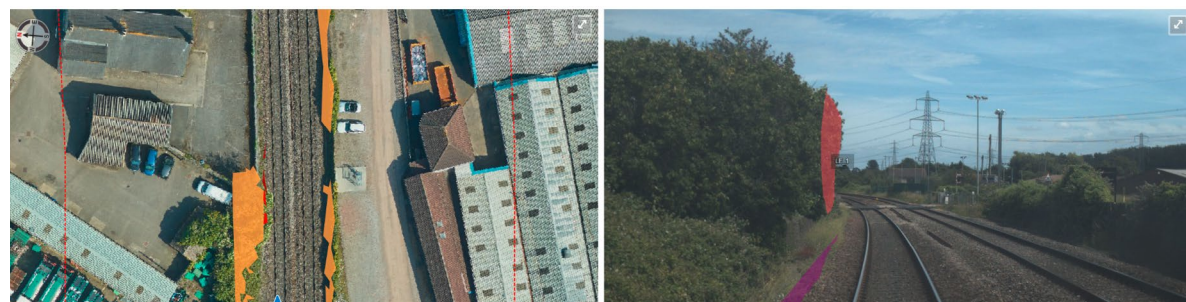
Figure 1 On the left, a top-down image of a railway line with encroaching vegetation highlighted in orange and red. On the right, a front on image of a railway line with encroaching vegetation highlighted in red and purple.
