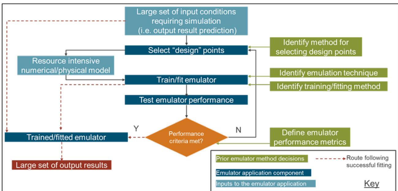
**Figure 1: Conceptual diagram of components of an emulator (key: green boxes - prior emulator method decisions; royal blue boxes - emulator application component; pale blue boxes - inputs to the emulator application; red dashed line – route following successful fitting)**
