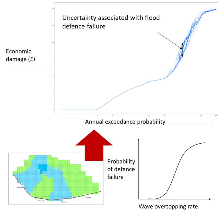
**Figure 26: Illustration of the stages involved in the Environment Agency's NaFRA coastal flood risk analysis. Two emulators are applied: one for wave transformation and the other for wave overtopping**
