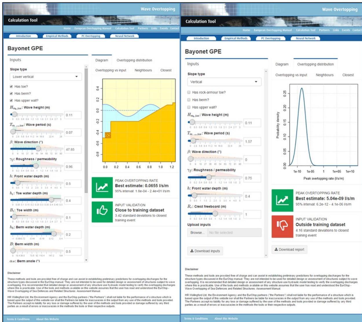
Figure 20: Screenshot of a translation of the Mahalanobis distance measure user guidance within an online wave overtopping model (source: <https://www.overtopping.co.uk>)
