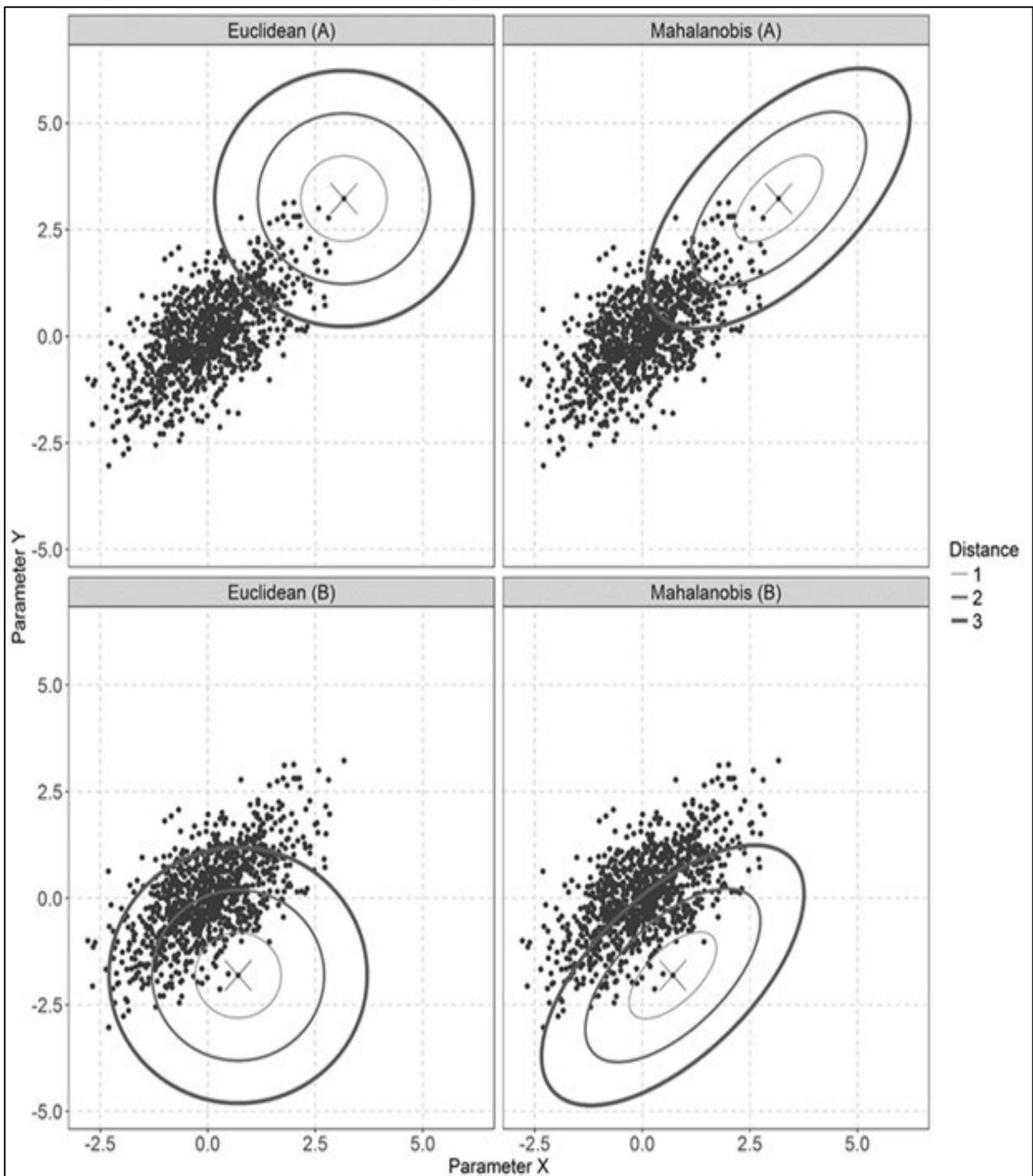
**Figure 19: Graphical illustration of the Mahalanobis distance measure, used to assess the limits of applicability of a wave overtopping emulator (source: Pullen and others, 2018)**
