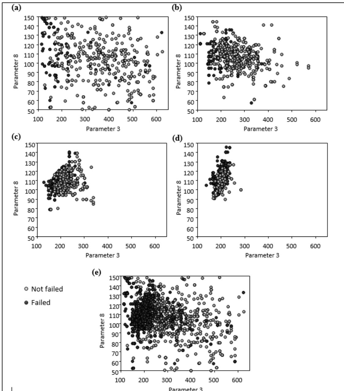
**Figure 15: Iterative selection of design points for an emulator of a geotechnical flood defence failure model, New Orleans (source: Kingston and others, 2011)**
