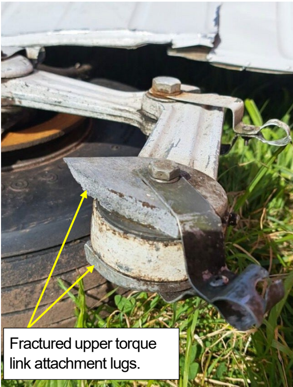
Detached torque link lugs and wheel assembly
