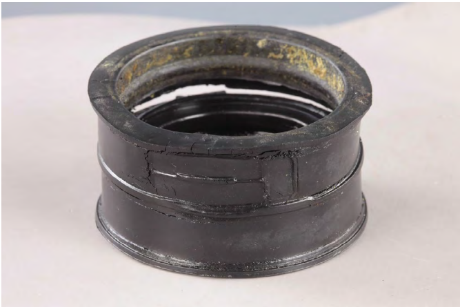
Split carburettor coupling from G-CDFK
