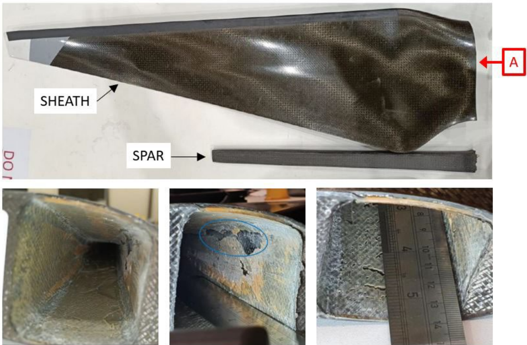
Released propeller blade including failed spar-to-sheath adhesive bond (lower three images, viewed in direction ‘A’) (courtesy of manufacturer)
