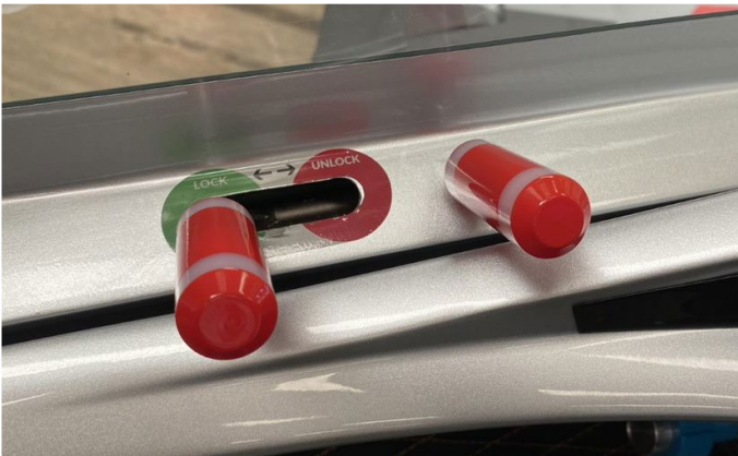
Shoot bolt handles (canopy in the closed and locked position)
