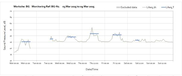
Note: Missing data between 18:00 on Monday 3<sup>rd</sup> March and 14:00 on Tuesday 4<sup>th</sup> March was due to a loss power to the monitoring station caused by poor weather conditions preventing sufficient light reaching the solar panel.
