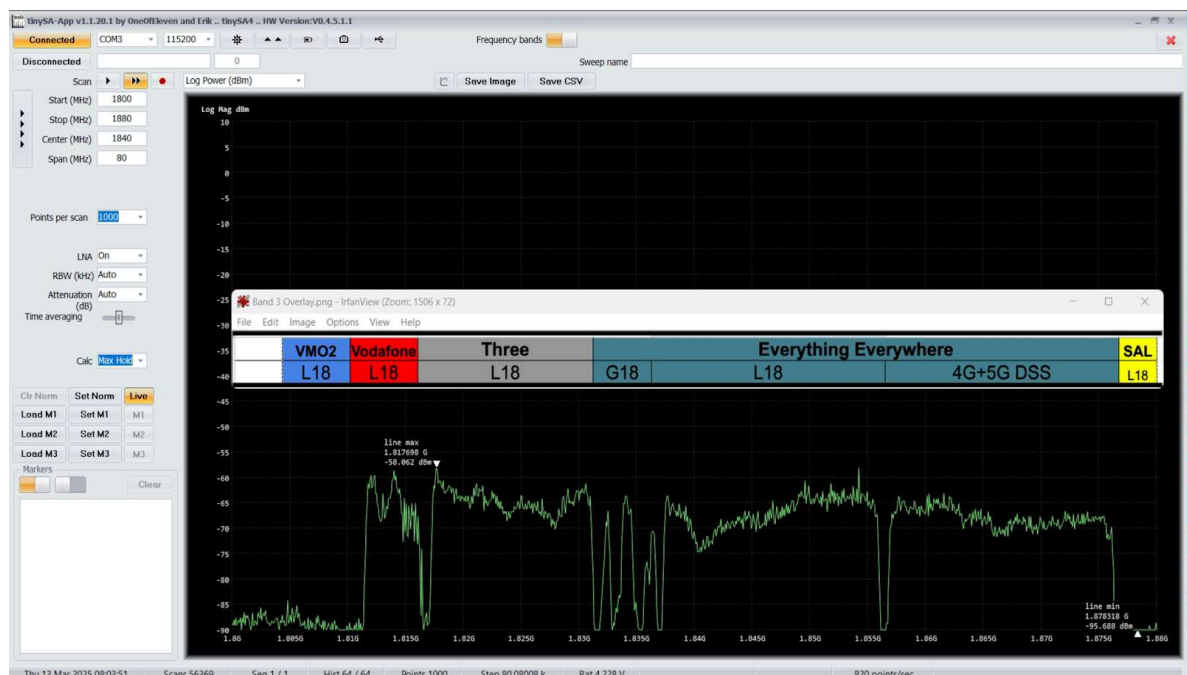
Figure 36: Example spectrum analyser plot showing the RF environment including the test radio operation. Occupied channels in the Three and EE spectrum allocations are clearly visible. Our DSA gNB is using a 5 MHz channel in the Vodafone allocation.
