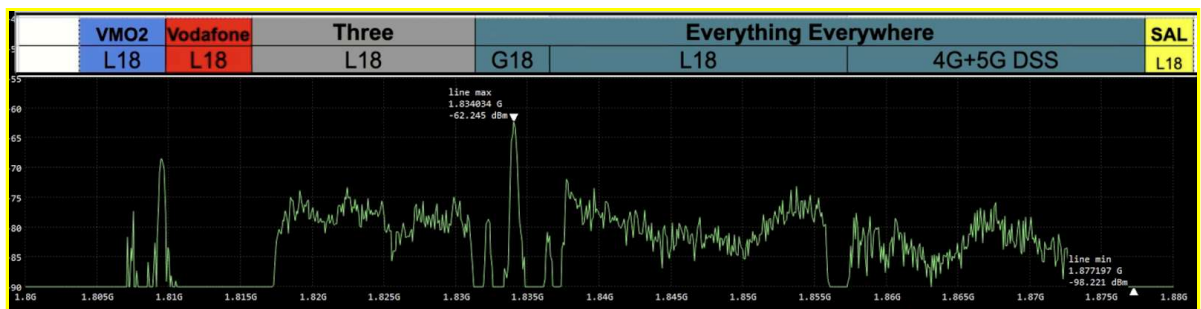
Figure 37: Co-channel interference is identified within 2 seconds of a MNO illuminating within their primary allocated spectrum. This causes the secondary user to release the channel and undertake a full band scan to collect full band spectrum occupancy, prior to submitting a new spectrum application to the DSA Server.
