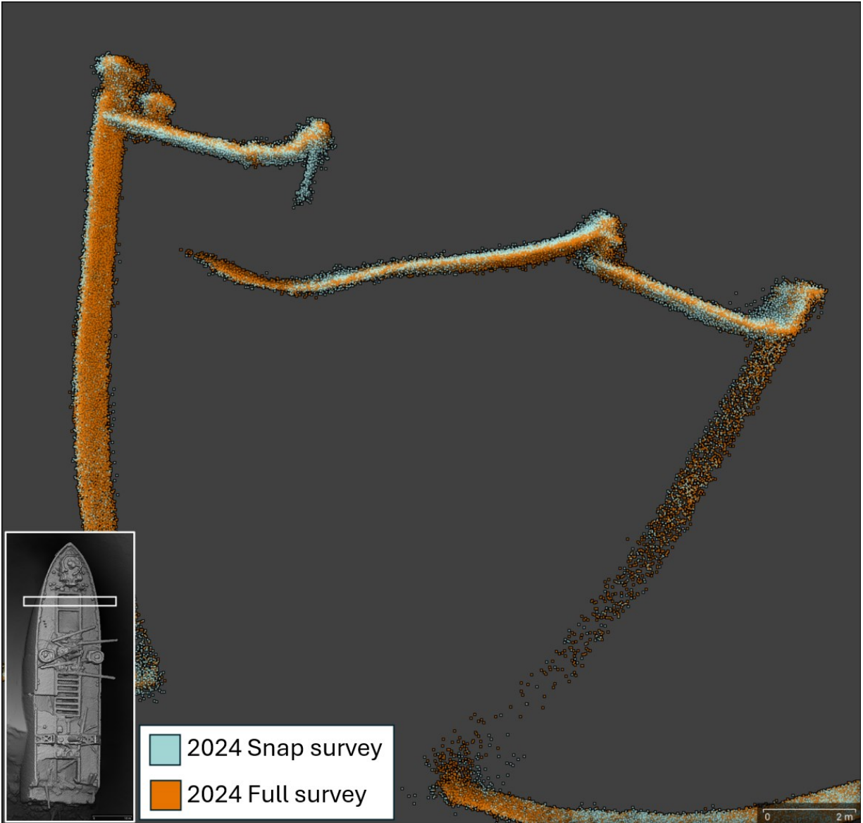
Figure 23. Cross section through the hull at the forward end of hold 1.
