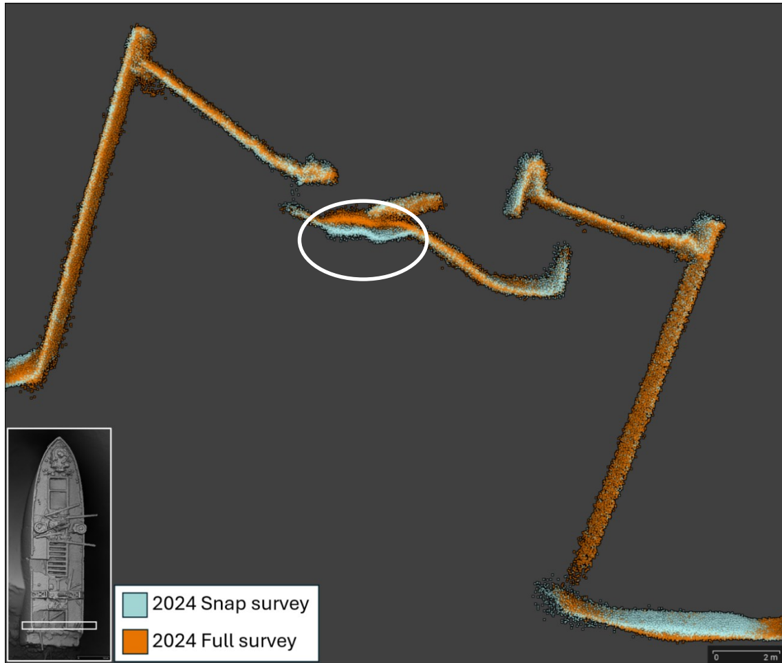
Figure 28. Cross section through the hull at the middle of hold 3. Difference in sediment level circled.
