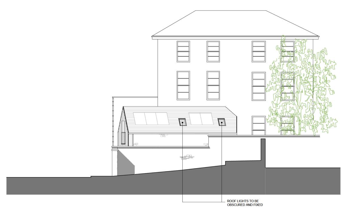
MATERIAL CLADDING MATERIALS: NEW STONE TO MATCH EXISTING GARDEN WALL BLUE SEMI-ENGINEERING BRICKS FOR PLINTH WESTERN RED CEDAR CLADDING TREATED WITH OSMO UV RESISTANT OIL WINDOWS: VELFAC 200 SERIES IN RAL 7015 RAINWATER GOODS: ALUMINIUM PROFILES IN RAL 7015
