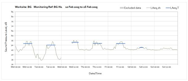
Note: Missing data between 00:00 and 10:00 on Wednesday 12<sup>th</sup> February was due to a loss of power to the monitoring station caused by poor weather conditions preventing sufficient light reaching the solar panel.
