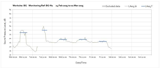
Note: Missing data between 07:00 and 11:00 on Tuesday 25<sup>th</sup> February was due to a loss of power to the monitoring station caused by poor weather conditions preventing sufficient light reaching the solar panel.
