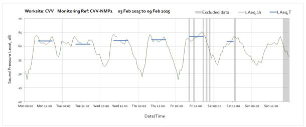
Note: Missing data between 13:00 and 15:00 on Tuesday  $4^{th}$  February was due to monitor maintenance. Missing data between 11:00 and 12:00 on Wednesday  $5^{th}$  February was due to a transmission error between the monitoring station and server.
