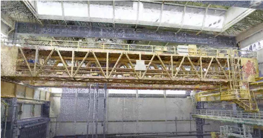
Photograph 15: LiDAR model of a section of the Turbine Hall
