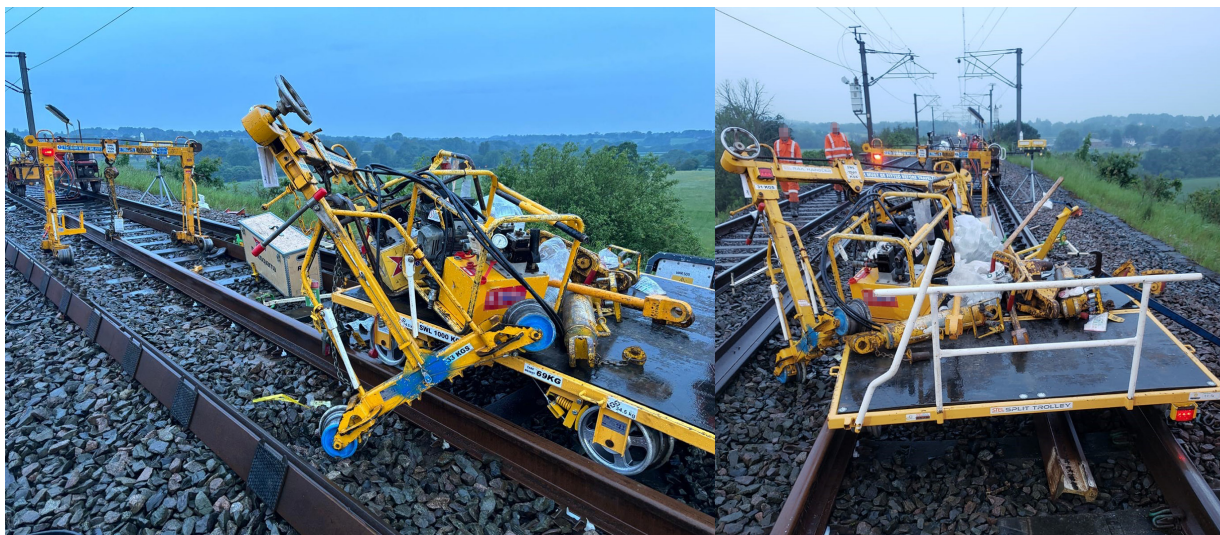
Figure 2: Final position of the runaway trolley having collided with the ironman (courtesy of Rhomberg Sersa Rail Group Ltd).
