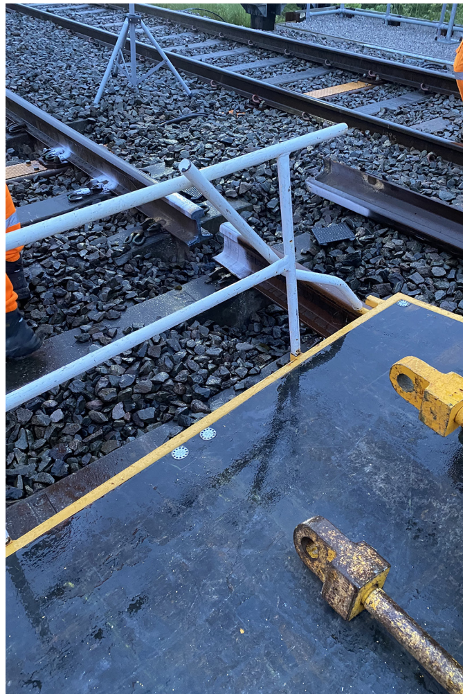
Figure 10: The brake handle, shown wedged under the push barrier, immediately after the collision (courtesy of RSRG).
