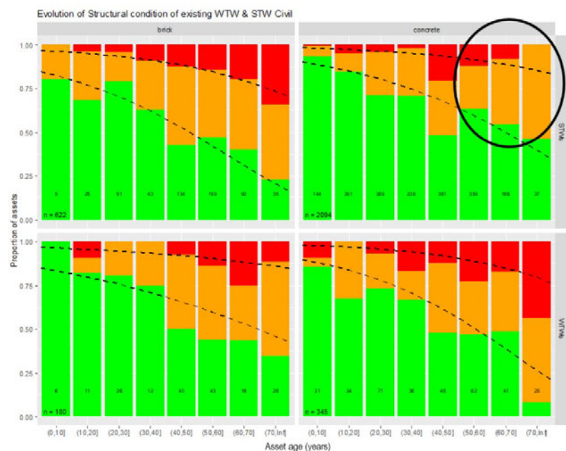
Figure 65: Northumbrian Water deterioration model outputs 47
