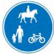
Figure 11-19 Diagram 956.1 (S3-2-30) Route for use by pedal cycles, horses and pedestrians only
