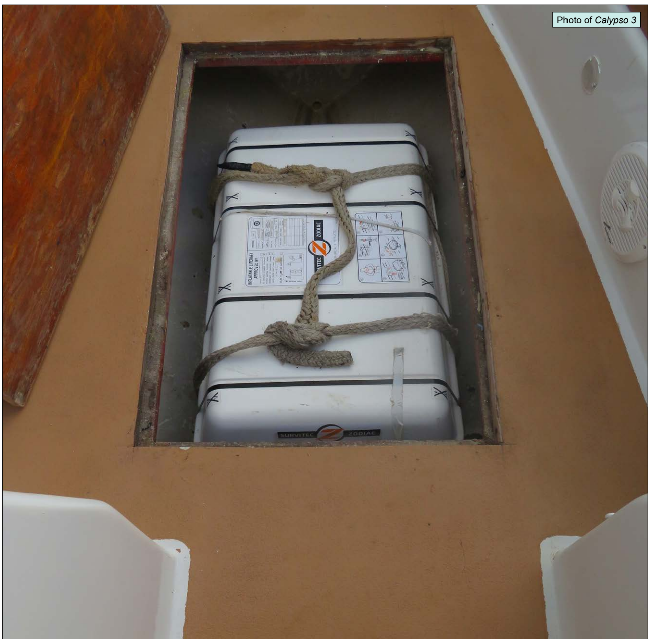
Figure 8: Liferaft stowage in the foredeck seating area
