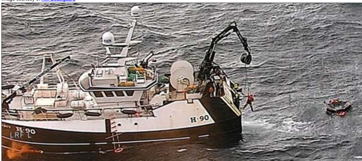
HM Coastguard helicopter footage following the collision, showing the overturned liferaft and a member of Guiding Star 's crew being recovered from the water using Guiding Light 's power block
