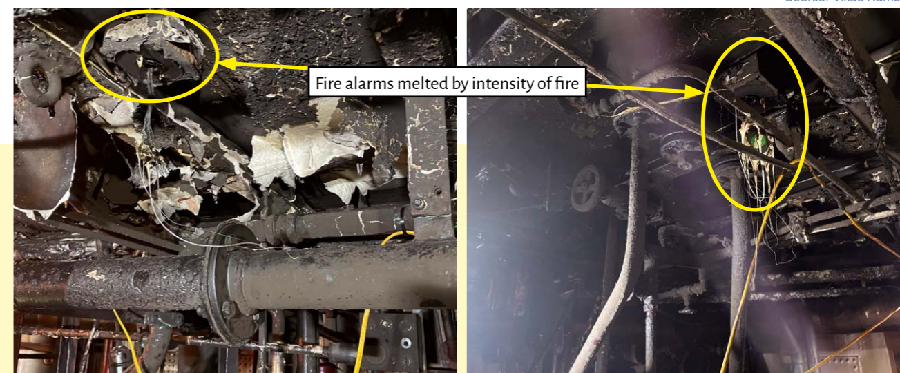
Figure 2: Smoke blackened deckhead and the remains of the fire alarms
