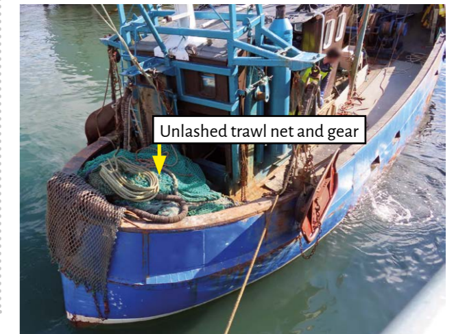
Figure: Net stowed at stern after the accident
