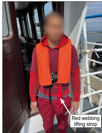
Figure: The red webbing lifting strop on the PFD
