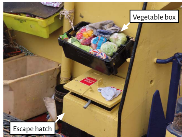
Figure 1: The blocked escape hatch
