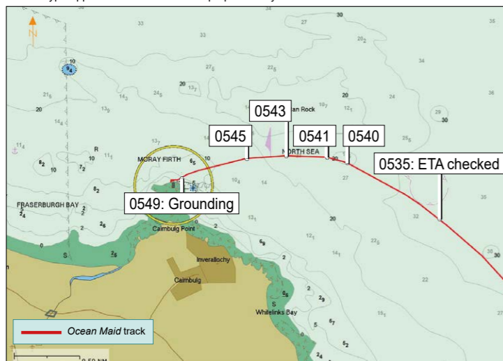
Figure: Chart showing the four course alterations leading up to the grounding
