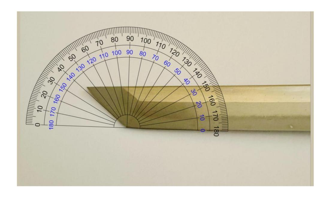
In this second photo with the protractor, the angle between the secondary straight cutting edge and the blunt spine of the blade is approximately 47 degrees (under 90 degrees).
