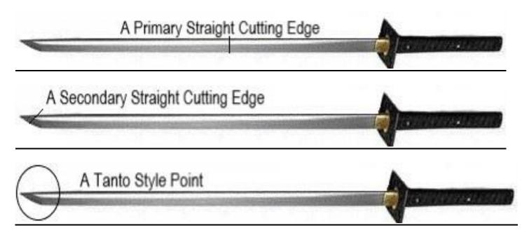
\*Note a tanto style point has angle of greater than 90 degrees between its primary straight cutting edge and its secondary straight cutting edge, and the angle between its secondary straight cutting edge and the blunt spine is an angle of less than 90 degrees.
