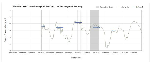
Note: Missing data between the start of the month and 12:00 on Tuesday 21<sup>st</sup> January was due to a loss of power to the monitoring station caused by poor weather conditions preventing sufficient light reach the solar panel.
