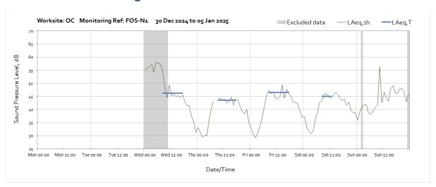
Note: Missing data between 08:00 and 09:00 on Thursday 2<sup>nd</sup> January was due to a loss of power to the monitoring station caused by poor weather conditions preventing sufficient light reach the solar panel.
