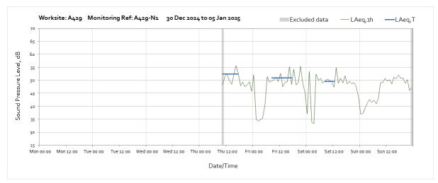
Note: Missing data between the start of the month and 09:00 on Thursday 2<sup>nd</sup> January was due to a loss of power to the monitoring station caused by poor weather conditions preventing sufficient light reach the solar panel.
