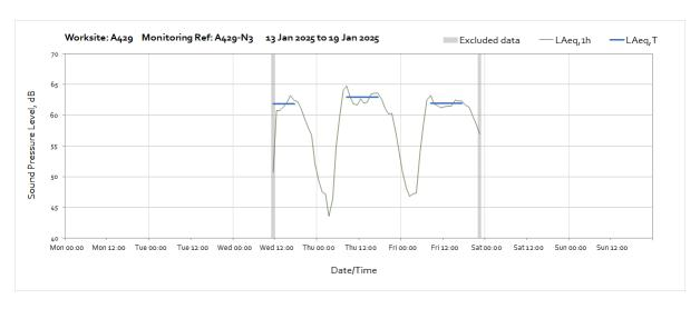
Note: Missing data throughout the month was due to a loss of power to the monitoring station caused by poor weather conditions preventing sufficient light reach the solar panel.
