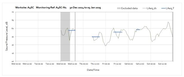
Note: Missing data between 16:00 on Wednesday 01<sup>st</sup> January and 08:00 on Thursday 02<sup>nd</sup> January was due to a loss of power to the monitoring station caused by poor weather conditions preventing sufficient light reach the solar panel.
