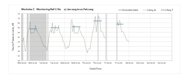
Note: Missing data between 23:00 on Thursday 30<sup>th</sup> January and 09:00 on Friday 31<sup>st</sup> January was due to a loss of power to the monitoring station caused by poor weather conditions preventing sufficient light reach the solar panel.
