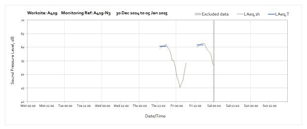
Note: Missing data throughout the month was due to a loss of power to the monitoring station caused by poor weather conditions preventing sufficient light reach the solar panel.
