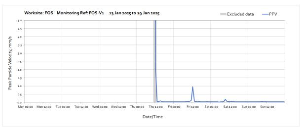
Note: Missing data between the start of the month and 10:00 on Thursday 16<sup>th</sup> January was due to a loss of power to the monitoring station caused by poor weather conditions preventing sufficient light reach the solar panel.
