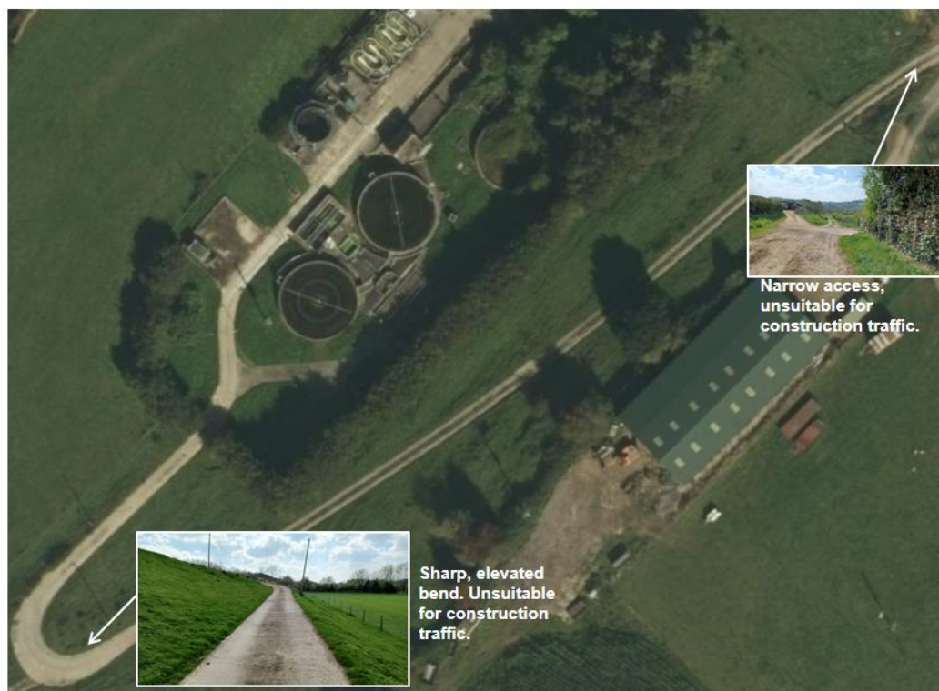
Figure A13-1 – Beckington WRC access track considerations
