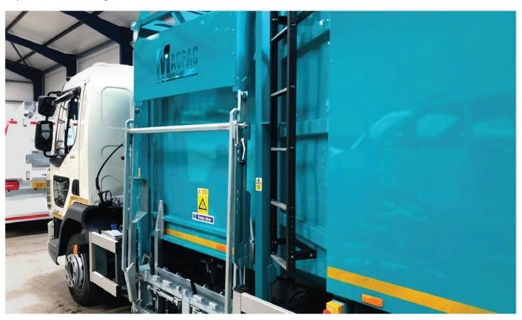
Toploader<sup>®</sup> side lifting mechanism.
