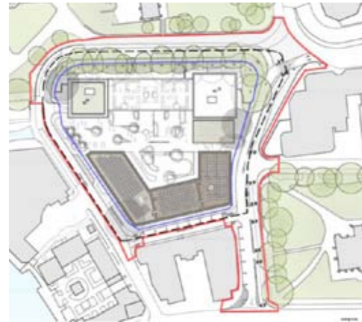
Figure 15: Measuring site areas (worked example using the recently consented Ambulance Station development)
