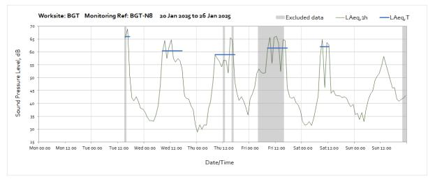
Note: Missing data between the start of the month and 14:00 on Tuesday 21<sup>st</sup> January was due to a loss of power to the monitoring station caused by poor weather conditions preventing sufficient light reach the solar panel.
