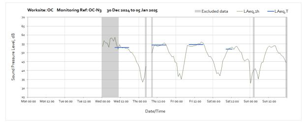
Note: Missing data bewteen 05:00 and 07:00 on Thursday 2<sup>nd</sup> January was due to a loss of power to the monitoring station caused by poor weather conditions preventing sufficient light reach the solar panel.
