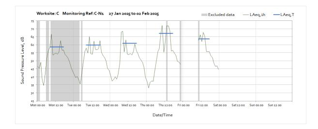
Note: Missing data between 23:00 on Thursday 30<sup>th</sup> January and 09:00 on Friday 31<sup>st</sup> January was due to a loss of power to the monitoring station caused by poor weather conditions preventing sufficient light reach the solar panel.
