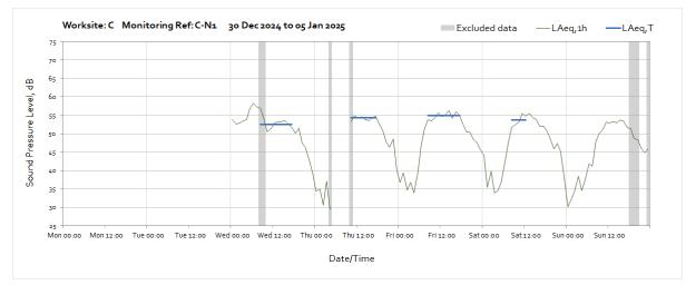
Note: Missing data between 05:00 and 09:00 on Thursday 2<sup>nd</sup> January was due to a loss of power to the monitoring station caused by poor weather conditions preventing sufficient light reach the solar panel.
