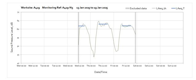
Note: Missing data throughout the month was due to a loss of power to the monitoring station caused by poor weather conditions preventing sufficient light reach the solar panel.
