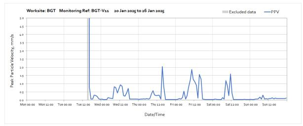
Note: Missing data between the start of the month and 14:00 on Tuesday 21<sup>st</sup> January was due to a loss of power to the monitoring station caused by poor weather conditions preventing sufficient light reach the solar panel.
