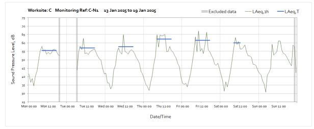
Note: Missing data between 20:00 on Monday 13<sup>th</sup> January and 05:00 on Tuesday 14<sup>th</sup> January was due to a loss of power to the monitoring station caused by poor weather conditions preventing sufficient light reach the solar panel.
