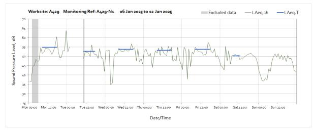
Note: Missing data between 02:00 and 09:00 on Tuesday 7<sup>th</sup> January was due to a loss of power to the monitoring station caused by poor weather conditions preventing sufficient light reach the solar panel.
