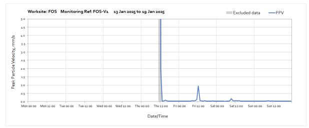
Note: Missing data between the start of the month and 10:00 on Thursday 16<sup>th</sup> January was due to a loss of power to the monitoring station caused by poor weather conditions preventing sufficient light reach the solar panel.
