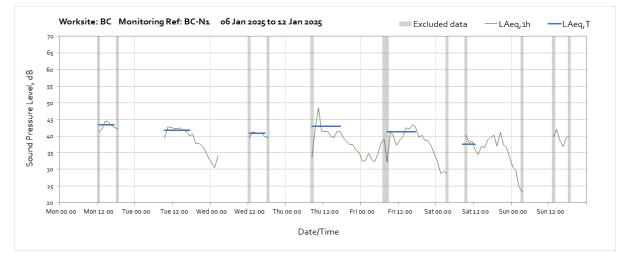
Note: Missing data throughout the month was due to a loss of power to the monitoring station caused by poor weather conditions preventing sufficient light reach the solar panel. OFFICIAL
