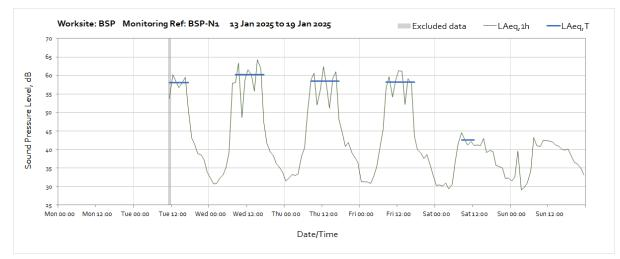
Note: Missing data between the start of the month and 10:00 on Tuesday 14<sup>th</sup> January was due to a loss of power to the monitoring station caused by poor weather conditions preventing sufficient light reach the solar panel.
