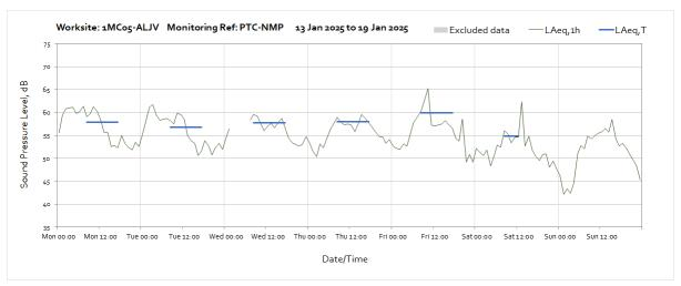
Note: Missing data between 02:00 and 06:00 on Wednesday 15<sup>th</sup> January was due to a loss of power to the monitoring station caused by poor weather conditions preventing sufficient light reach the solar panel.
