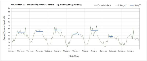
Note: Missing data between 15:00 and 16:00 on Tuesday 14<sup>th</sup> January was due to a communication error between the monitoring station and server.
