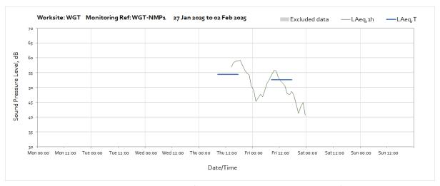
Note: Missing data between 18:00 on Friday 24<sup>th</sup> January until 14:00 on Thursday 30<sup>th</sup> January was due to a damaged battery cable causing a depleted monitor battery.
