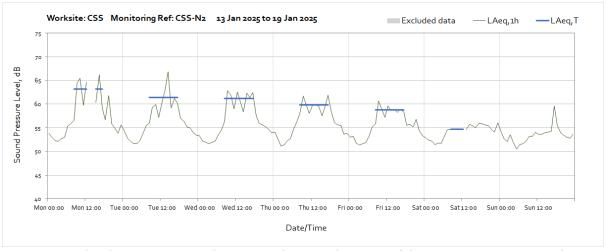
Note: Missing data between 13:00 and 15:00 was due to replacement of the noise monitor. Missing data between 09:00 and 13:00 on Saturday  $18^{th}$  January was due to power supply issues on site.
