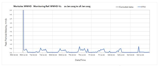
Note: Missing data between the beginning of the month and 11:00 on Monday 20<sup>th</sup> January was due to a loss of power to the monitoring station caused by poor weather conditions preventing sufficient light reaching the solar panel.
