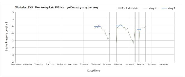
Note: Missing data throughout the week was due to a loss of power to the monitoring station caused by poor weather conditions preventing sufficient light reaching the solar panel.
