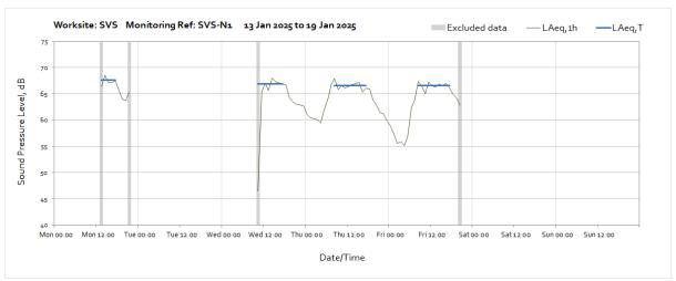
Note: Missing data throughout the week was due to a loss of power to the monitoring station caused by poor weather conditions preventing sufficient light reaching the solar panel.
