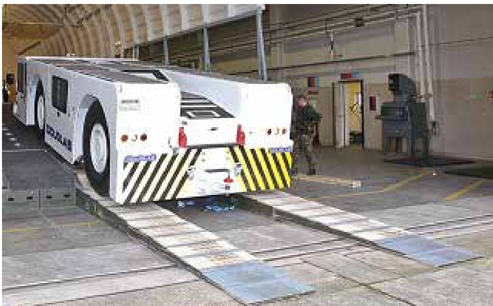
Figure 1 - Approach shoring used to reduce approach angle
