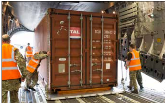
Image 3 & 4 - Transferring a 20 ft. ISO Container located on 463L air cargo pallet onto the C-17A - rollers configured for ADS.
