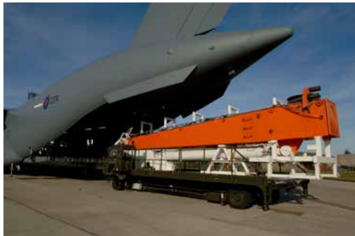
Image 1 - Palletised equipment loaded into a C-17A using an Atlas Transfer Loader
