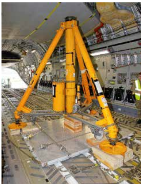
Image 2 - Aircraft jack in a C-17A - loaded on pallets
