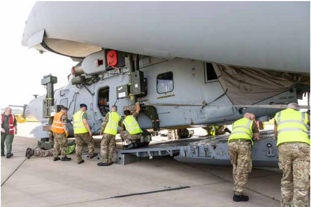
Image 10 - Merlin HC Mk 4 winched into a C-17A Globemaster
