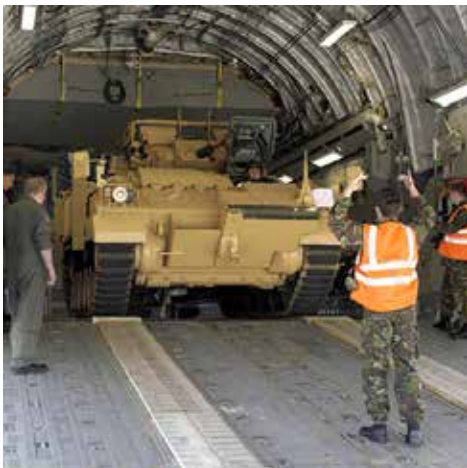
Image 1 - Warrior Armoured Tracked Vehicle on C-17A
