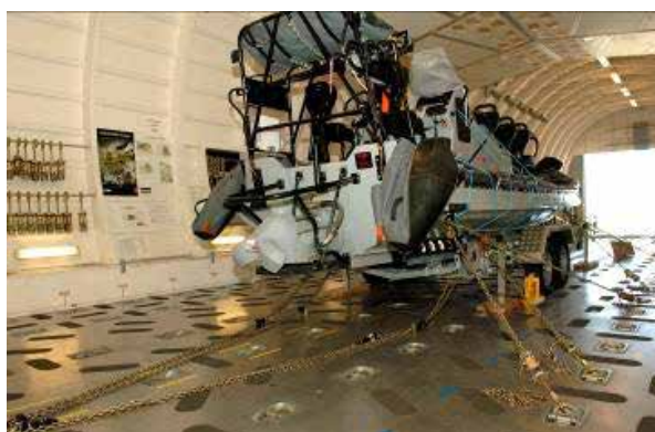
Image 2 - 24 ft. RIB and trailer individually restrained to the aircraft floor
