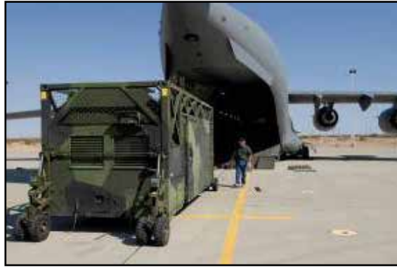
Image 9 - Cabin on mobilisers - to be winched into a C-17A
