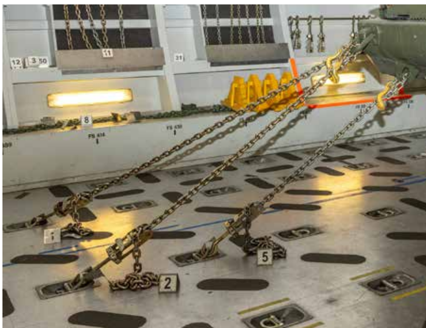
Figure 3 - C-17A – 25 000 lb. Tie down chains and tensioners
