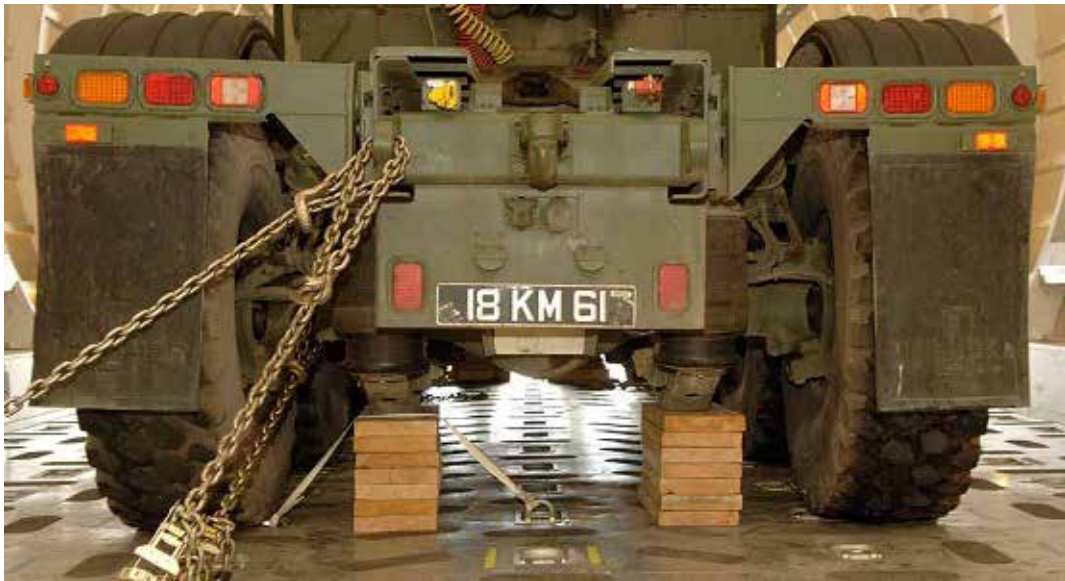
Figure 2 - Rear axle sleeper shoring using standard dunnage.
