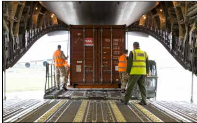
Image 3 & 4 - Transferring a 20 ft. ISO Container located on 463L air cargo pallet onto the C-17A - rollers configured for ADS.
