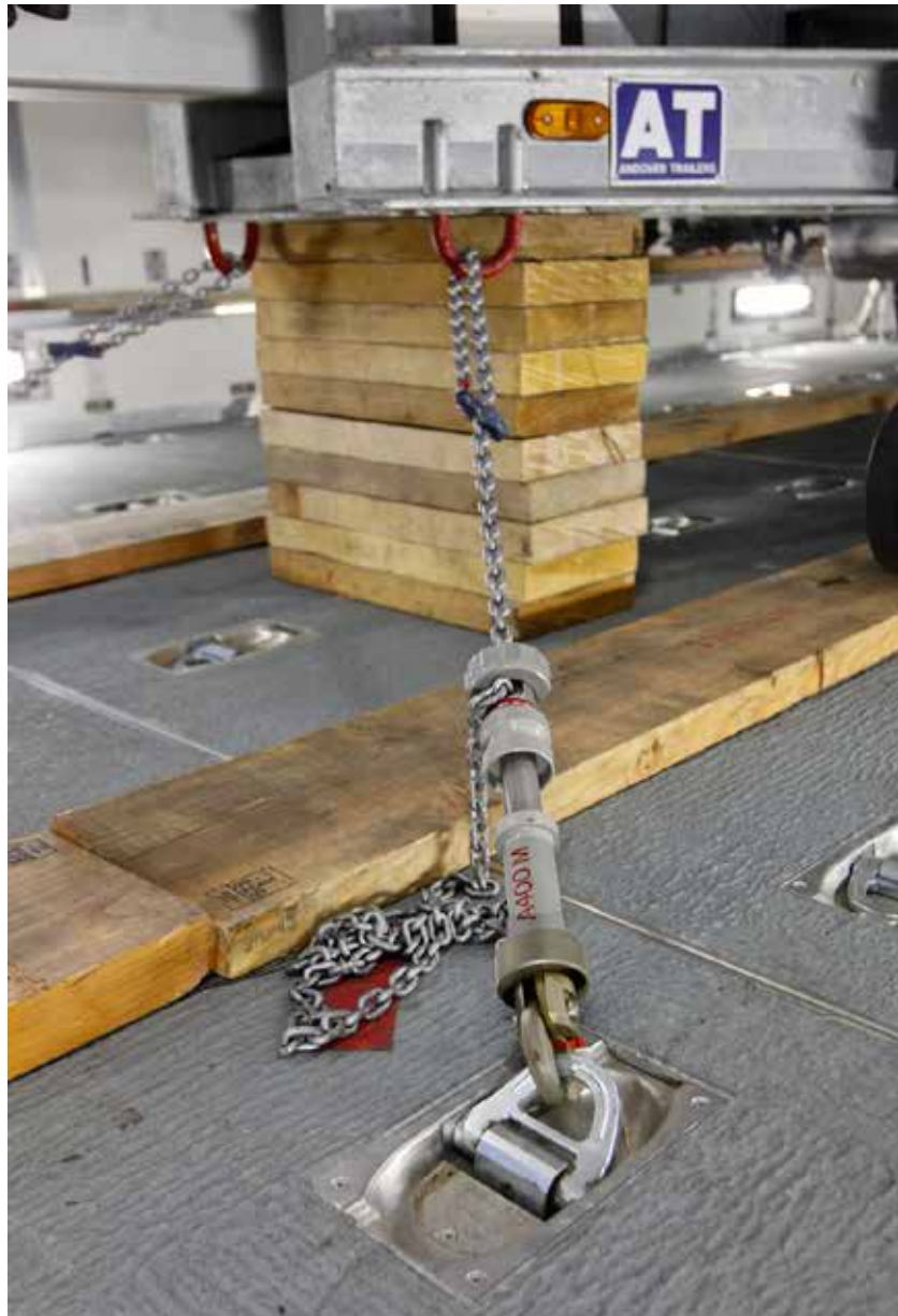
Figure 4 - A400M - 4535 kg. Tie down chain and tensioner
