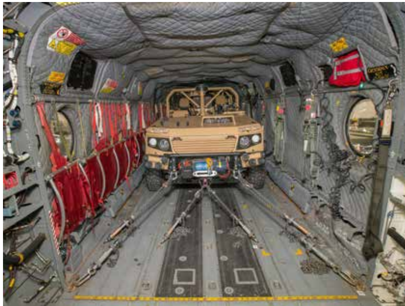
Image 8 - Vehicle restrained inside Chinook HC Mk 6
