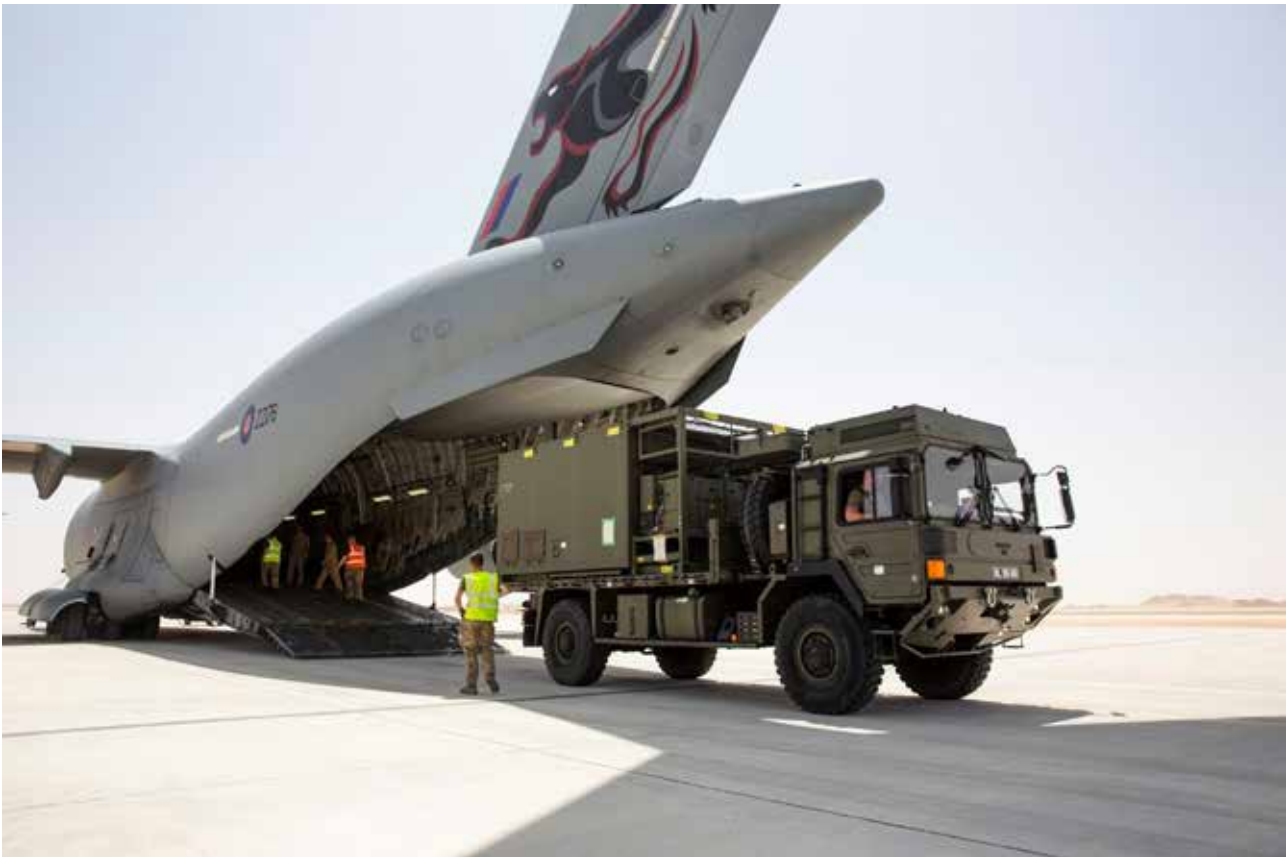
Figure 2 - C-17A - Loading a MAN SV.
