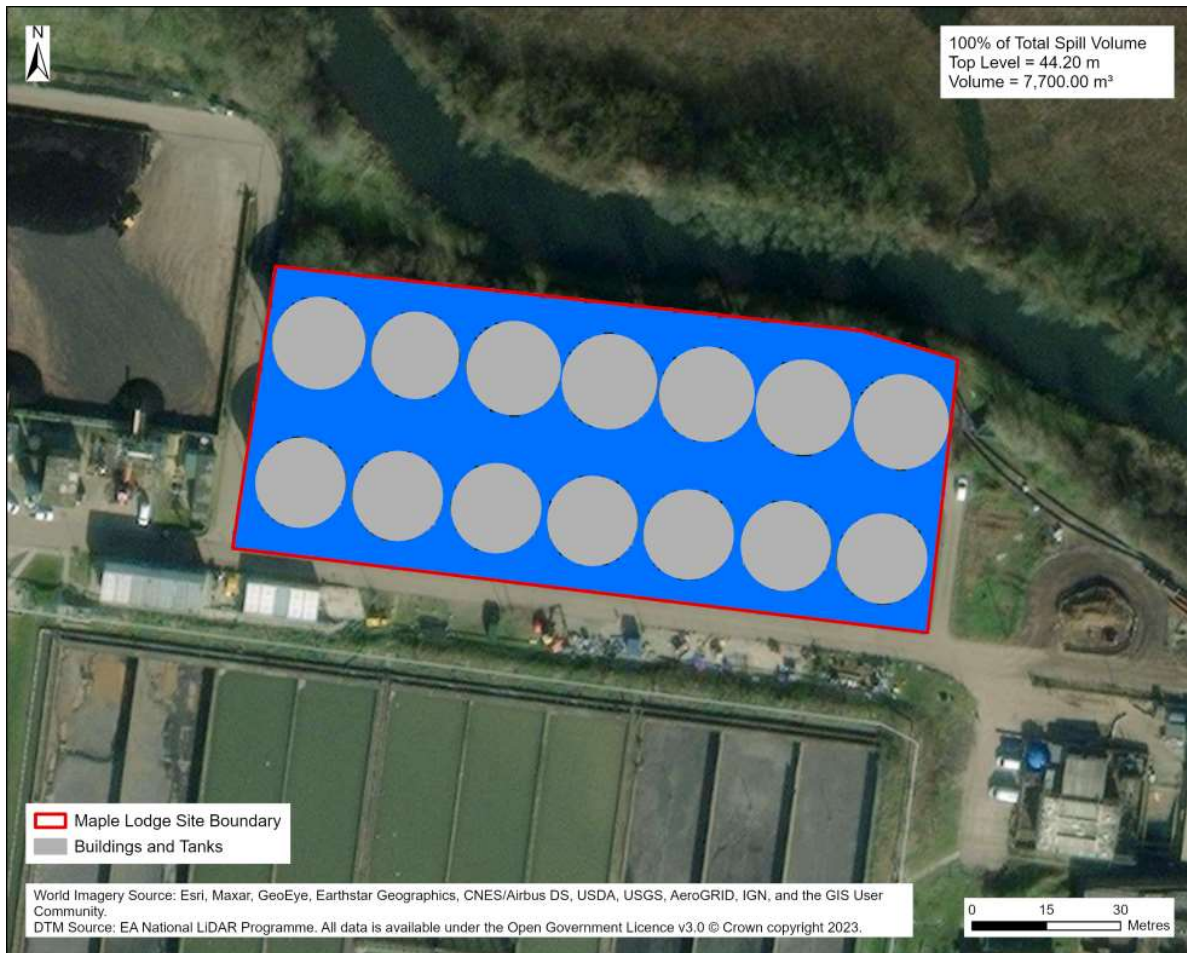
Figure 3-3 – Secondary Digesters area contained model
