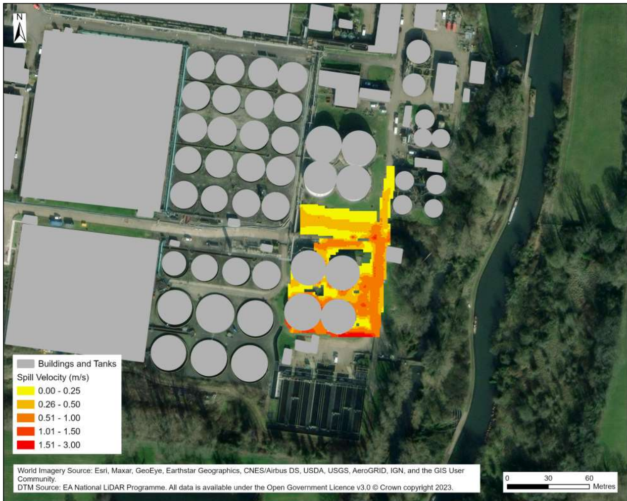
Figure 3-6 – Southern Primary Digesters area velocities
