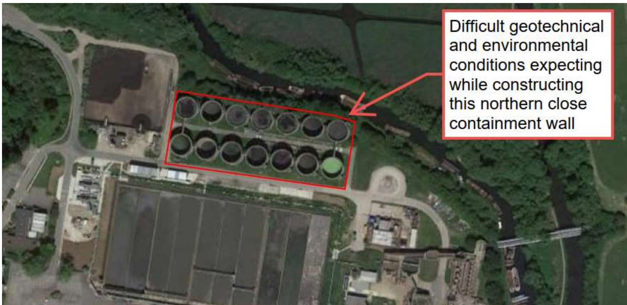
Figure 3-10 - Secondary Digester Environmental and Geotechnical Constraints
