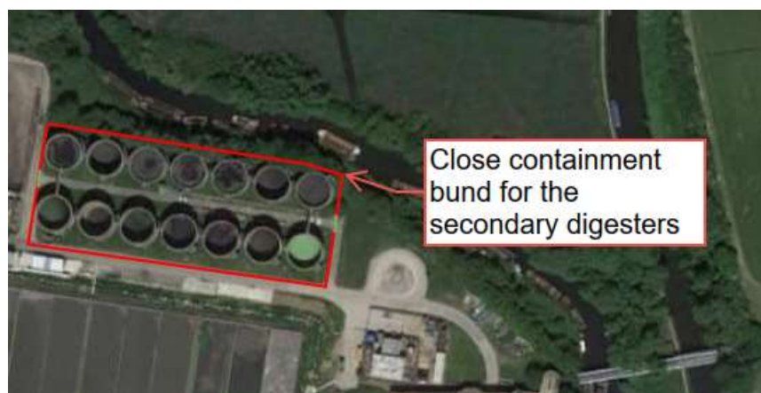
Figure 4-4 – Close Containment Bund for the Secondary Digesters
