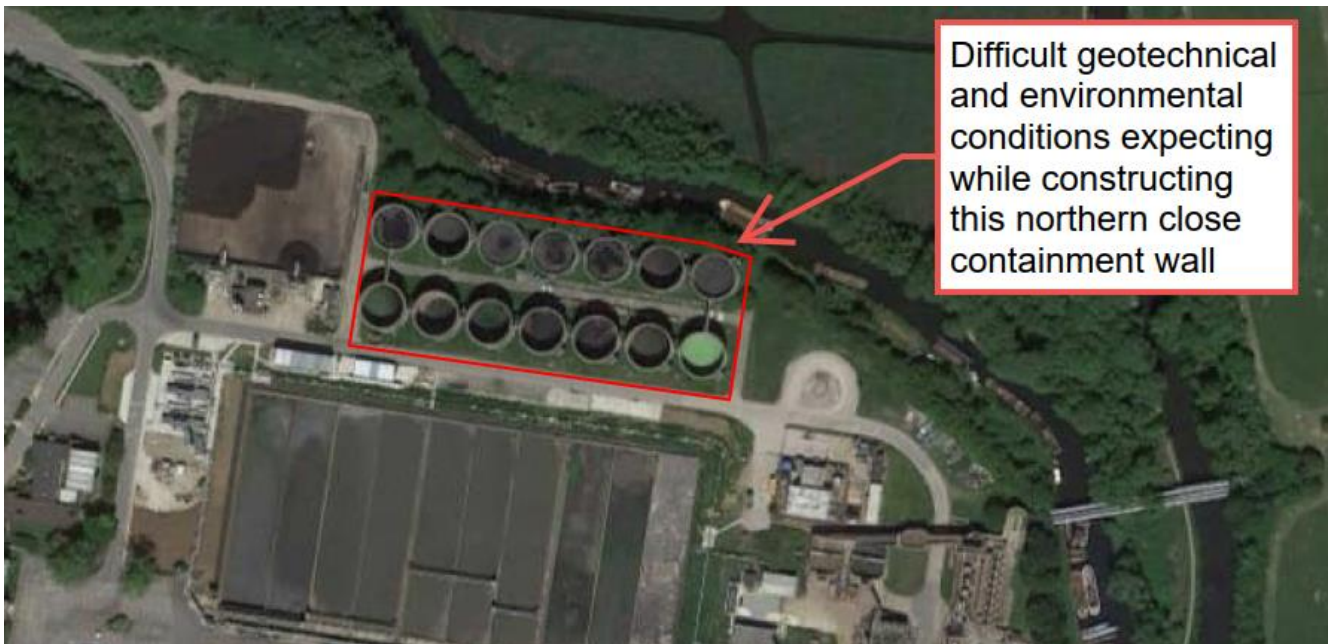
Figure 3-10 – Secondary Digester Environmental and Geotechnical Constraints
