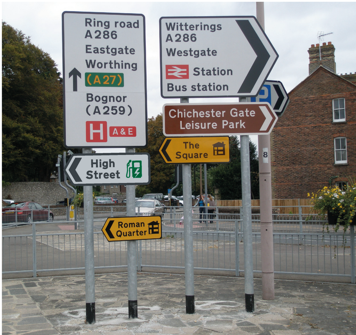
Fig. 19 D1. urban streetscape with one sign in a group containing an EV charging point symbol (here Symbol 1 in green).
