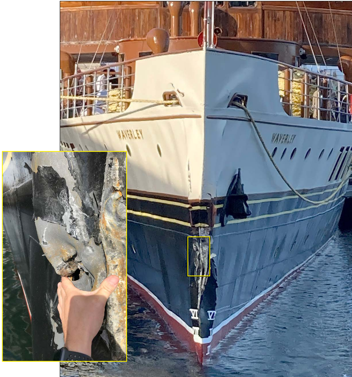
Figure 7: Damage sustained to the vessel's bow and the berth
