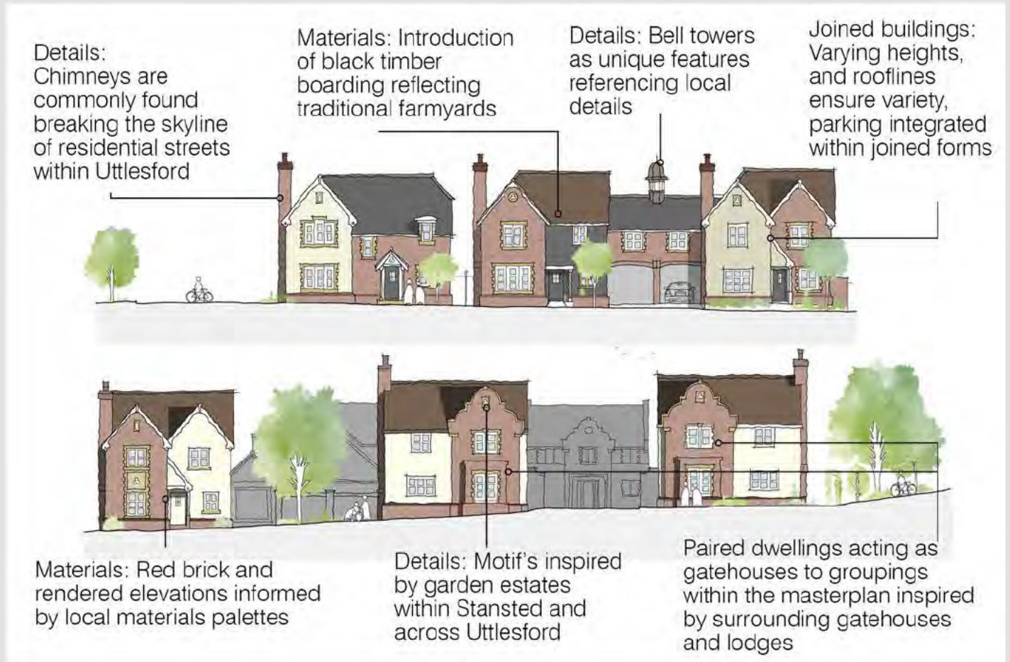
▲ Front elevation sketch of Dairy Lane, Stansted Mountfitchet. The sketch illustrates the ways it has interpreted local Uttlesford context.
