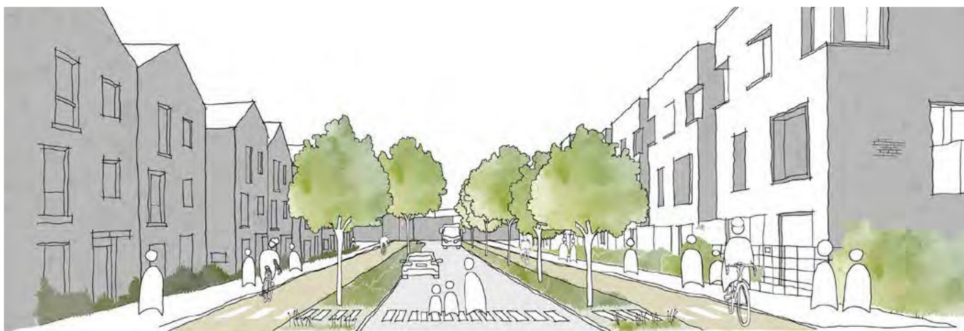
▲ Above is an illustrative sketch for a successful Market Street. It contains key features such as wide footways and cycle lanes on both sides of the street, and a range of SuDS and landscaping elements incorporated into the street scene.
