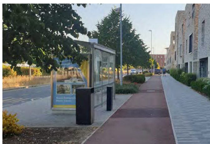
▲ Bus stops provided with suitable space to safely embark / disembark, whilst safely separated from the adjacent cycleway.
