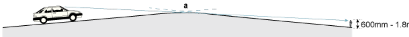
Forward visibility 25m in 20mph (30kph) zones; 43m on 30mph (50kph) roads a. Vertical curve at summit
