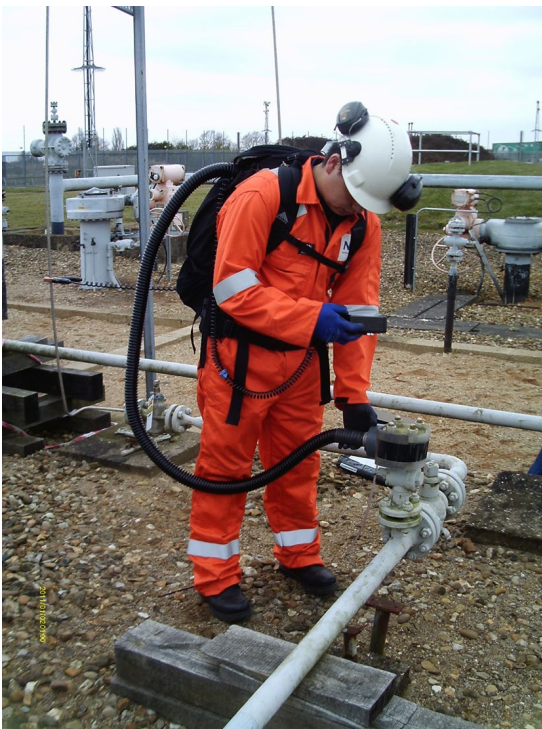
Figure 6: Photo of Bacharach Hi Flow® sampler in operation
