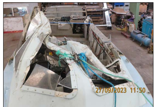
Figure 4: Lexi Rose post-recovery and damage to the deck
