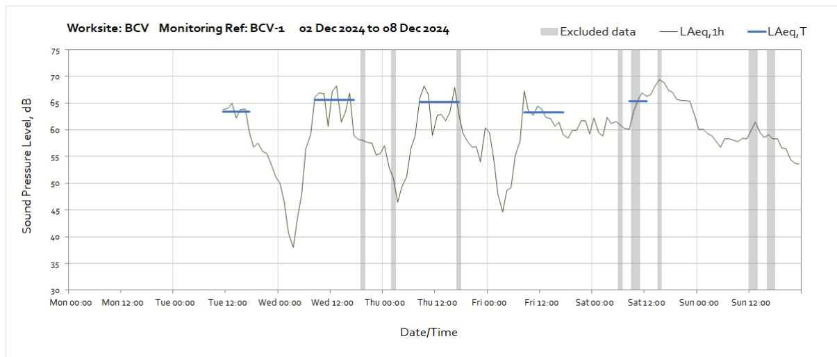
Note: Missing data from the beginning of December until 11:00 on Tuesday 3<sup>rd</sup> December was due to a loss of power to the monitoring station caused by poor weather conditions preventing sufficient light reaching the solar panel.
