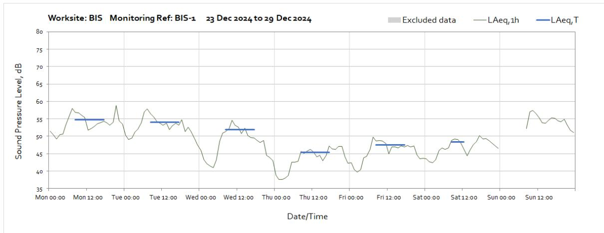
Note: Missing data between 00:00 and 08:00 on Sunday 29<sup>th</sup> December was due to a loss of power to the monitoring station caused by poor weather conditions preventing sufficient light reaching the solar panel.
