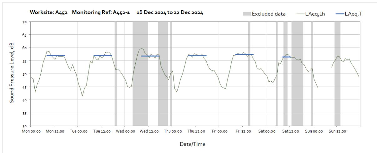
Note: Missing data between 03:00 and 09:00 on Sunday 22<sup>nd</sup> December was due to a loss of power to the monitoring station caused by poor weather conditions preventing sufficient light reaching the solar panel.
