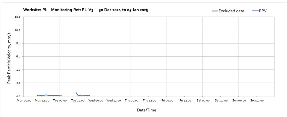
Note: Missing data throughout the month was due to a loss of power to the monitoring station caused by poor weather conditions preventing sufficient light reaching the solar panel.
