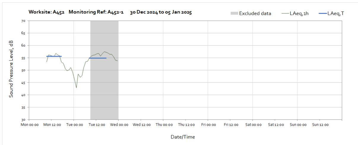
Note: Missing data between 20:00 on Sunday 29<sup>th</sup> and 09:00 on Monday 30<sup>th</sup> December was due to a loss of power to the monitoring station caused by poor weather conditions preventing sufficient light reaching the solar panel.
