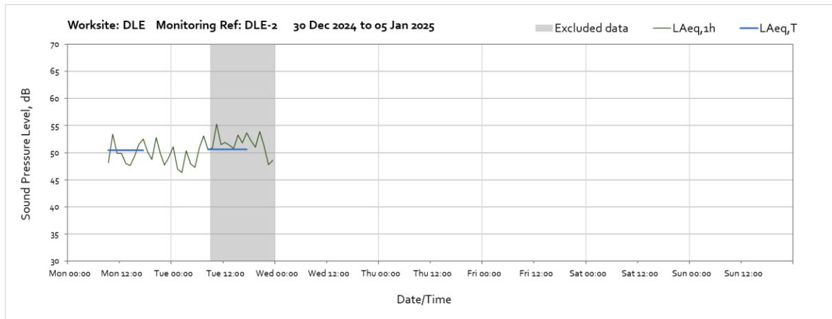
Note: Missing data between 18:00 on Sunday 29<sup>th</sup> and 09:00 on Monday 30<sup>th</sup> December was due to a loss of power to the monitoring station caused by poor weather conditions preventing sufficient light reaching the solar panel.
