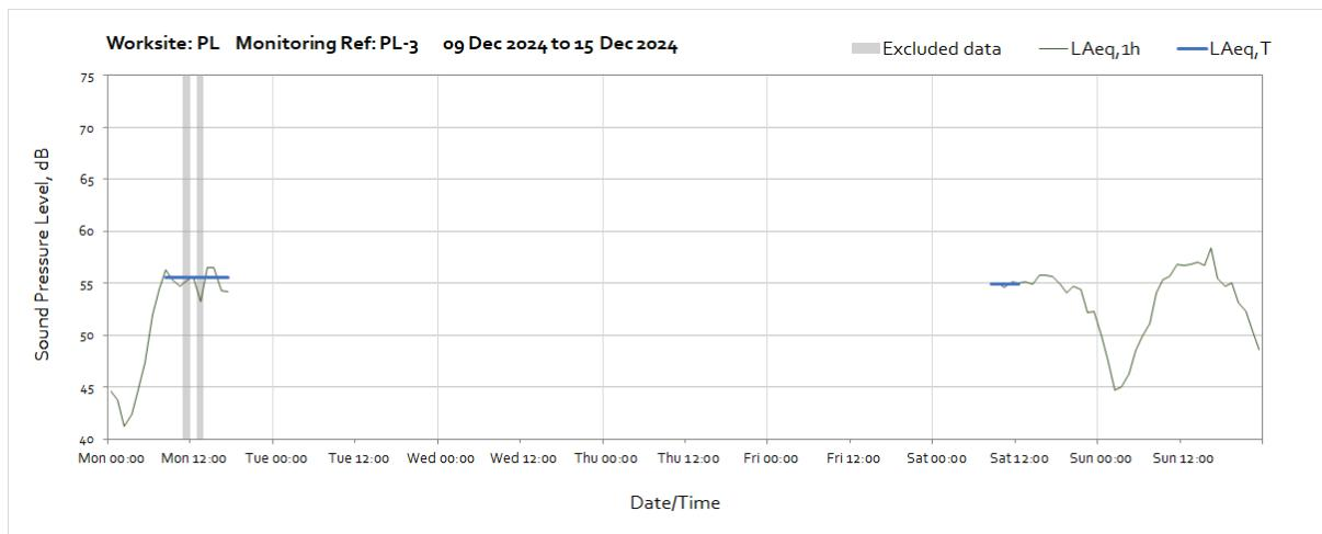
Note: Missing data throughout the month was due to poor solar conditions impacting power supply to the monitoring station.
