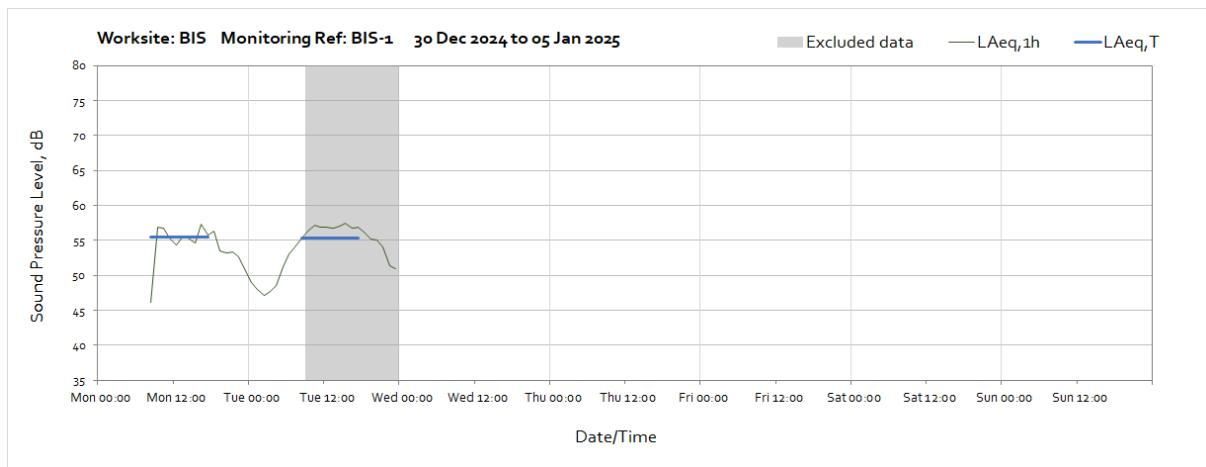
Note: Missing data between 00:00 and 08:00 on Monday 30<sup>th</sup> December was due to a loss of power to the monitoring station caused by poor weather conditions preventing sufficient light reaching the solar panel.
