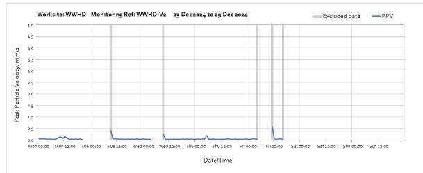
Note: Missing data throughout the week and to the end of the month was due to a loss of power to the monitoring station caused by poor weather conditions preventing sufficient light reach the solar panel.
