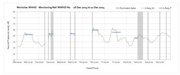
Note: Missing data throughout the week was due to a loss of power to the monitoring station caused by poor weather conditions preventing sufficient light reach the solar panel.
