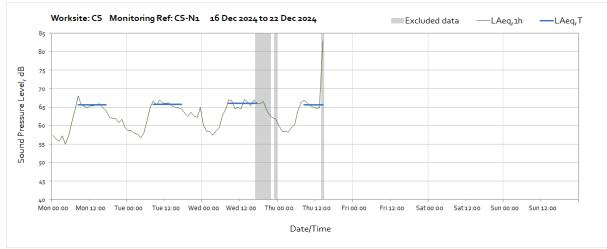
Note: Missing data between 15:00 on Thursday 19<sup>th</sup> December and the end of the month was due to noise monitor being removed for laboratory calibration.
