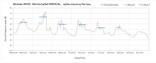
Note: Missing data between 08:00 and 09:00 on Saturday 14<sup>th</sup> December was due to a loss of power to the monitoring station caused by poor weather conditions preventing sufficient light reach the solar panel.
