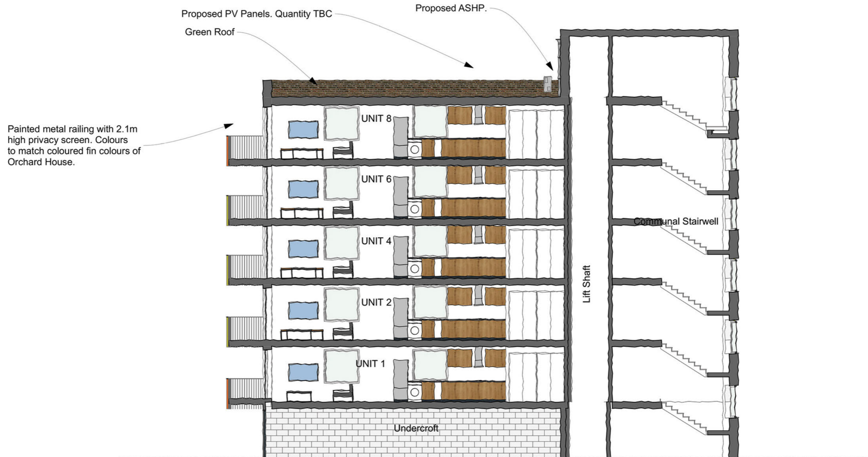
Building Section A-A Orchard House
