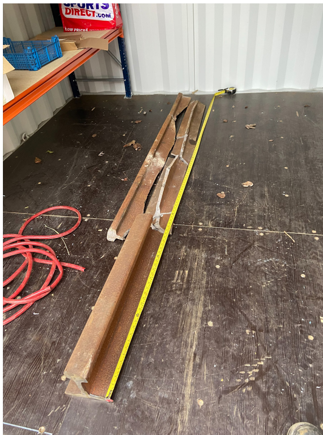
Figure 13: The section of running rail having been reassembled from the fragments found on and near the RRAP after the collision.
