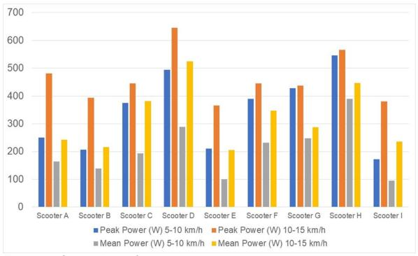
Figure 10: Comparison of calculated e-scooter power
