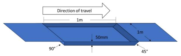
Figure 2: eKFV obstacle #1 - pothole with vertical entry and ramped exit
