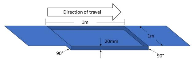
Figure 3: eKFV obstacle #2 - pothole with vertical entry and exit
