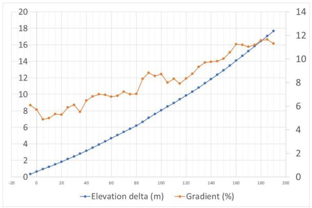
Figure 7: Surveyed elevation delta profile and calculated gradient
