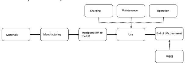
Figure 11 System boundary diagram for the LCA on shared e-scooters in the UK
