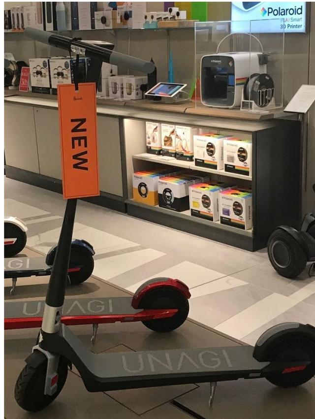
**Figure 1: Example of an e-scooter offered for sale in the UK, with a long single tube steering assembly and low frame**
