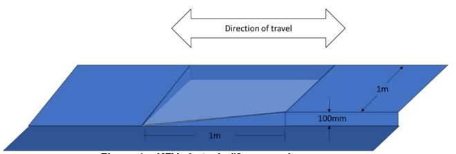
Figure 4: eKFV obstacle #3 - warped ramp
