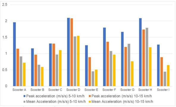
Figure 9: Comparison of measured e-scooter acceleration
