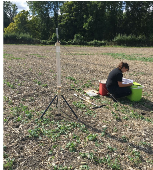
Figure 10. Measurements of soil hydraulic conductivity being taken on a controlled traffic field at Hendred Farm. Image credit: John Robotham.
