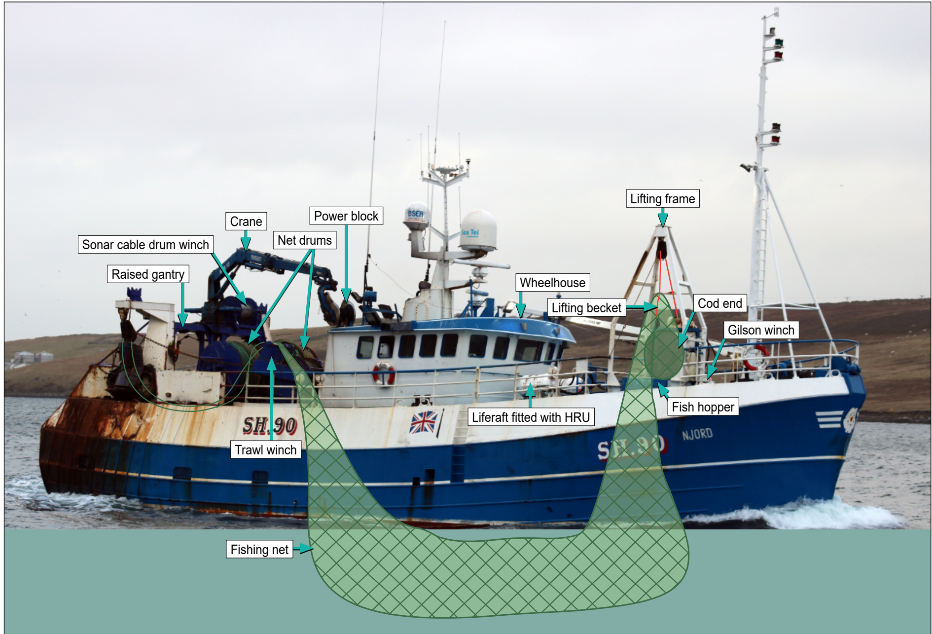
Figure 2: Njord net indicative lashing and general layout
