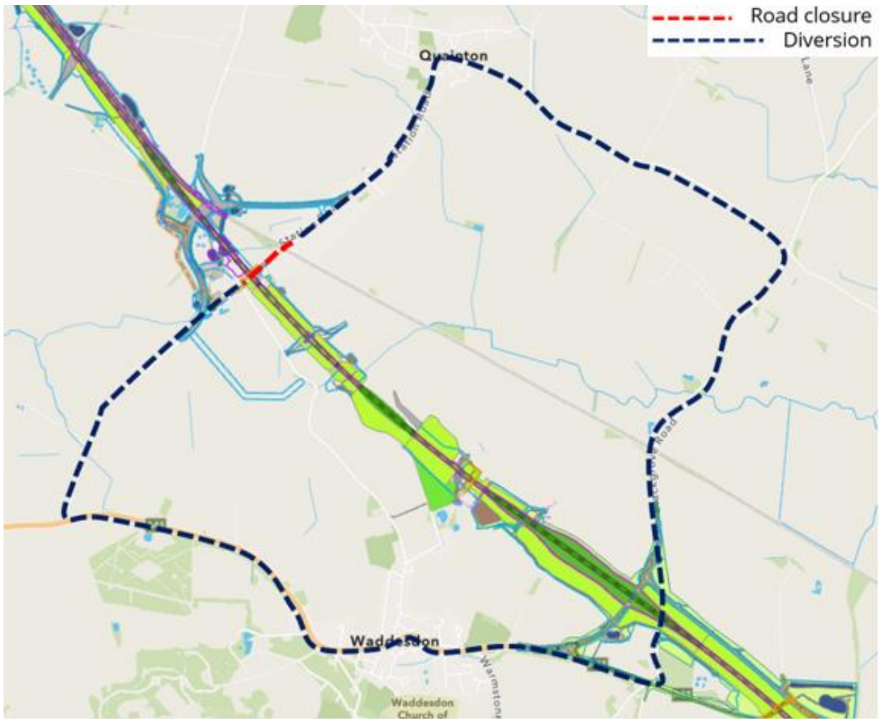
Figure A 4. Temporary closure of Station Road (east) and 11.4 km diversion
