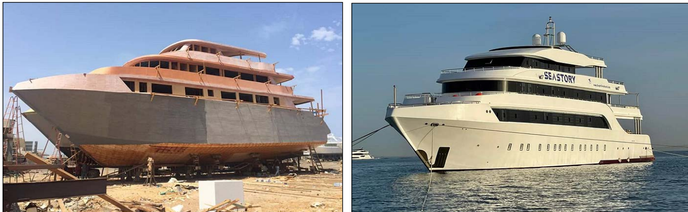
Figure 2: Sea Story before and after modification, including extension
