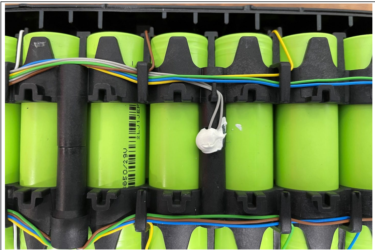
Figure 65: Voltage Sense Wire and Thermistor Wire Restraining Features in Product #6
