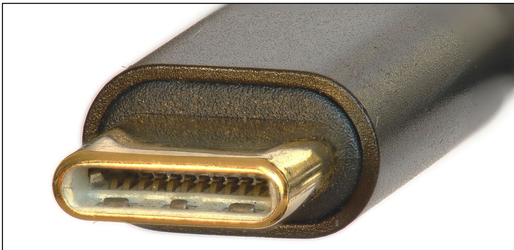
Figure 32: The USB-C (or USB Type-C) Connector
