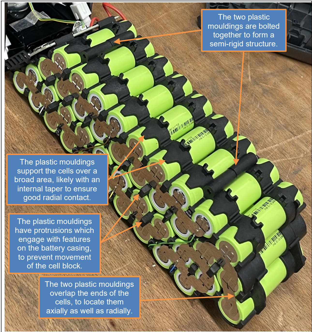
Figure 57: The Cell Support Structure in Product #6
