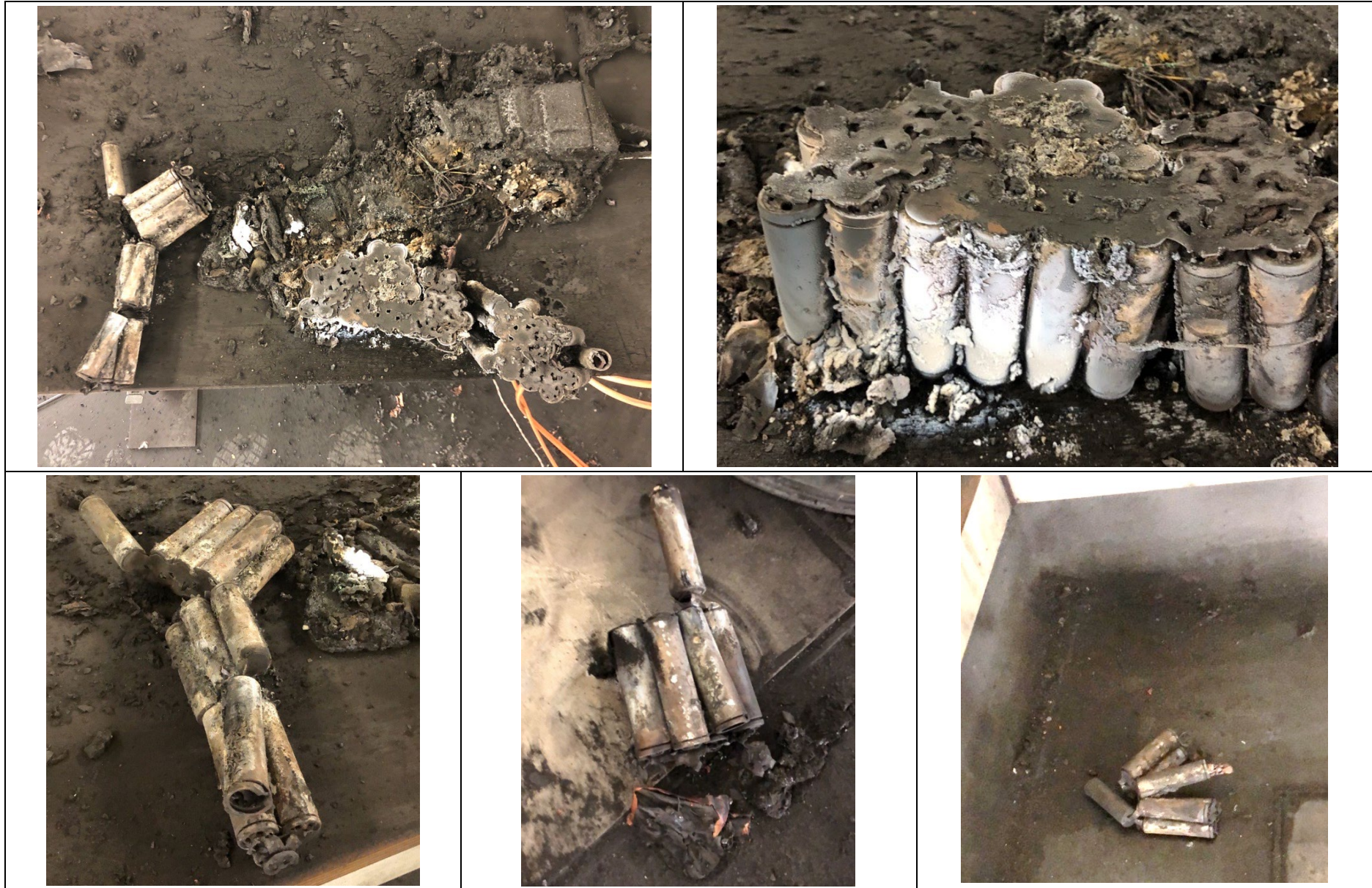
Figure 80: Photos of the Remains of Example 3 of Product #7, After Thermal Runaway
