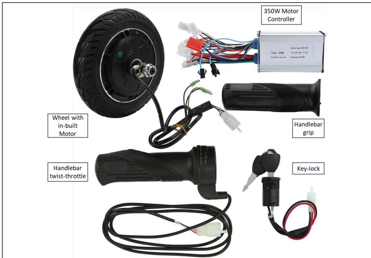
Figure 41: Example of e-scooter Conversion Kit, comprising a replacement wheel with in-built motor; a motor controller; replacement handlebar grips including a twist-throttle and a key-lock (Depisuta, no date)
