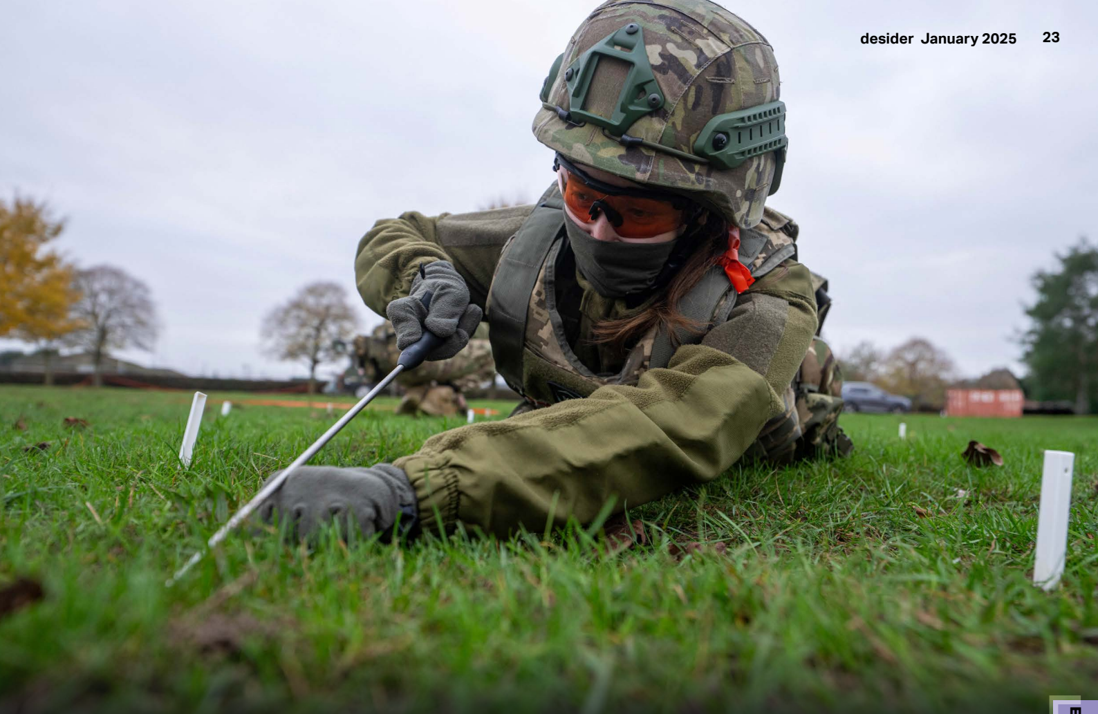
A member of the Armed Forces of Ukraine uses a compact landmine prodder to detect landmines during Explosive Ordnance Disposal training provided by the UK as part of Operation Interflex.
