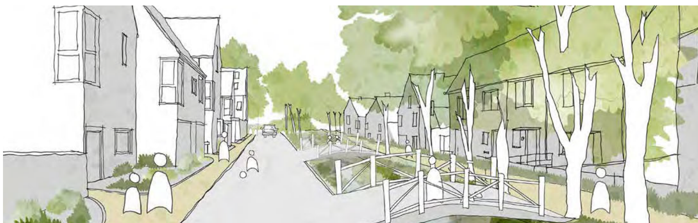
▲ A Village Street, as sketched above uses the existing landscape to structure the street. A footpath lined with mature trees runs parallel to the river, providing access to homes from the street. Slow vehicle speeds and narrow carriageways allow for informal play and social interaction.
