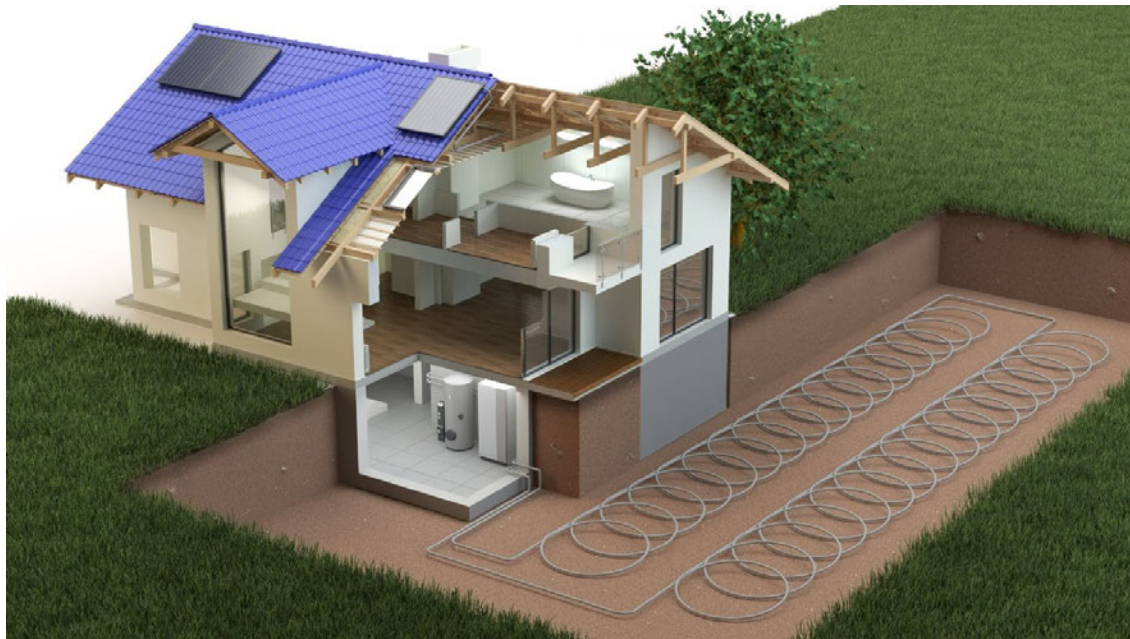
Horizontally sunk ground source heat pump
