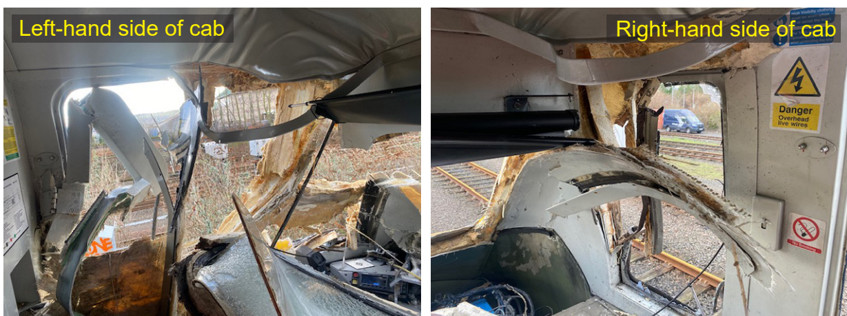
Figure 21: Internal damage sustained to leading power car of 1A37.
